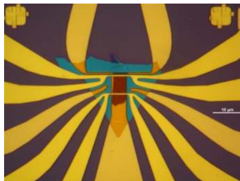
Figure 1: 2D material based device for electric and thermoelectric measurements
