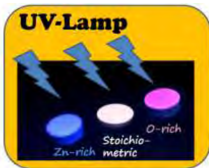
Figure 1. Defect evolution of non-stoichiometric ZnO.
