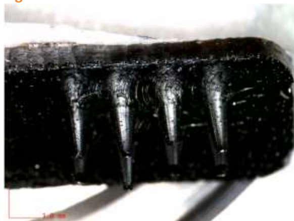
Figure 1. Graphene-based conductive coating on polymer microneedles
