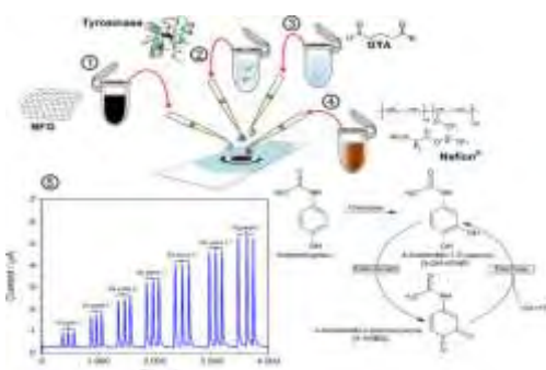
Figure 2. Preparation process of Tirosinase biosensor
