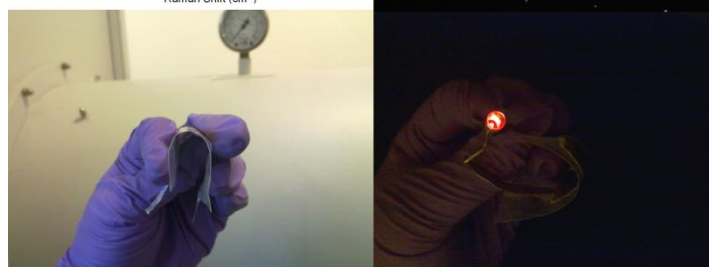
Figure 2. Monolayer graphene battery lights up LED
