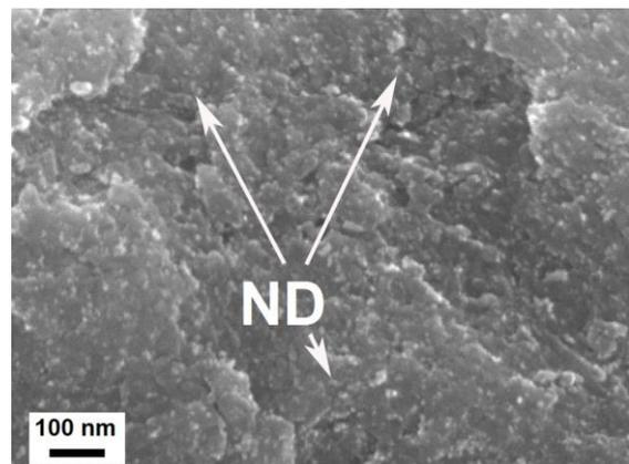
Figure 2. Granule surface of composite "Copper + nanodiamonds" after 4h treatment in planetary mill: arrows mark non-agglomerated nanodiamond particles
