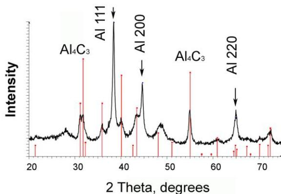
Figure 1. X-ray diffraction patterns from composite "Aluminum + nanodiamonds" after 8h treatment in planetary mill: vertical lines mark aluminum carbide peaks
