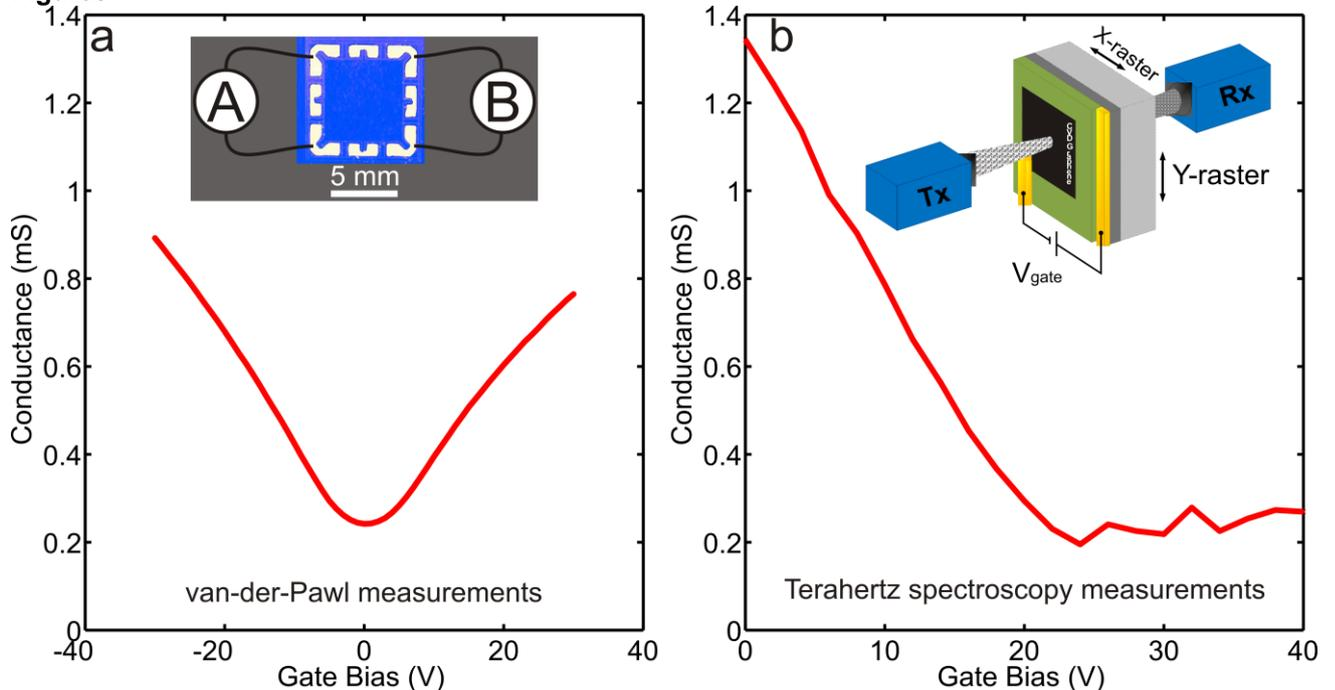
Figure 1: Gated measurements performed on mm<sup>2</sup>-sized areas of CVD graphene: a) using van der Pawl measurement technique with fixed gold electrodes. Inset: typical device with example of vdP circuit. b) using broadband transmission THz spectroscopy. Inset: schematic of terahertz setup showing gated measurements of graphene.
