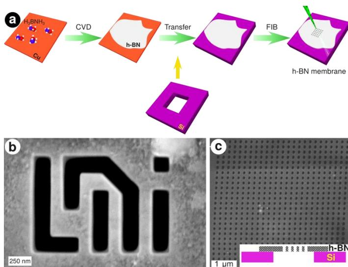
**Fig.** (a) Fabrication process of h-BN membranes. h-BN is first grown on copper foils, the copper is then etched in an ammonium persulfate solution. The floating h-BN film is transferred onto a hollow silicon substrate and patterned by FIB.
