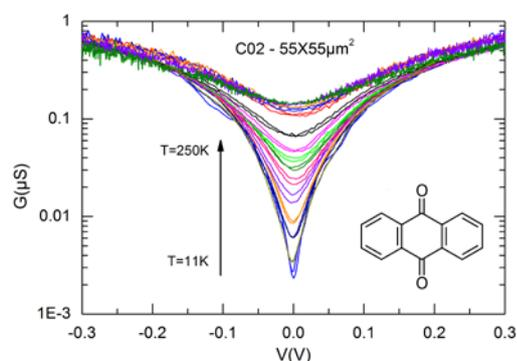
Measured conductance as a function of applied voltage of an anthraquinone based junction for temperatures varying between 11 k and 250 K.
