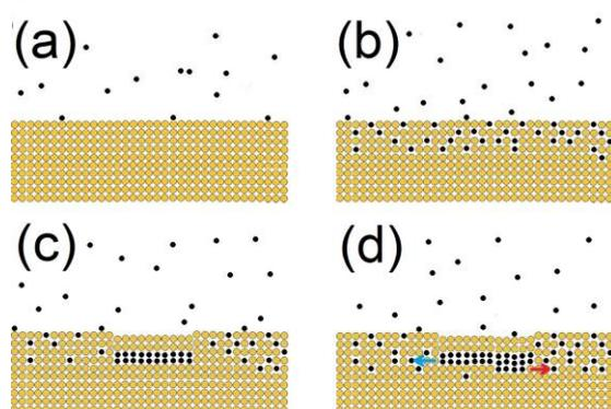
Fig.1 Process of subsurface nanoclusters formation. (a) Beginning of Co deposition on a hot Cu(001) substrate. (b) Incorporation and accumulation of Co in the near-surface region. (c) formation of an initial Co cluster. (d) Further growth of the next layer of the clusters, accompanied by Co segregation (blue and red arrows).
