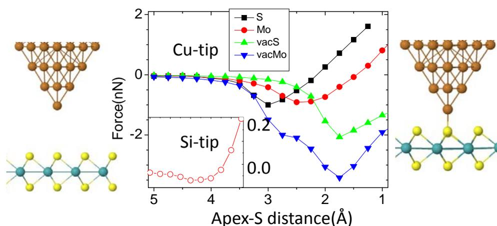
Figure 1: Schematic representation of a Cu tip over a S atom in the MoS<sub>2</sub> monolayer for long distance and in the contact regime together with the force curves obtained over the S and Mo atoms and their corresponding vacancies. In the inset, the same result obtained over a Mo atom using a low interacting Si-tip.
