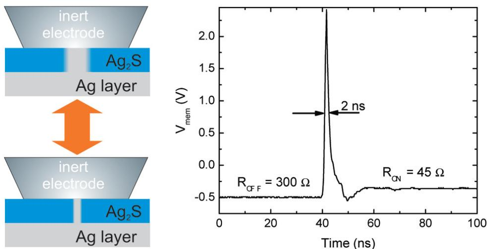
**Fig.1** Resistive switching taking place at nanosecond timescales in the Ag<sub>2</sub>S layer are attributed to a change in the diameter of the metallic conducting channel.
