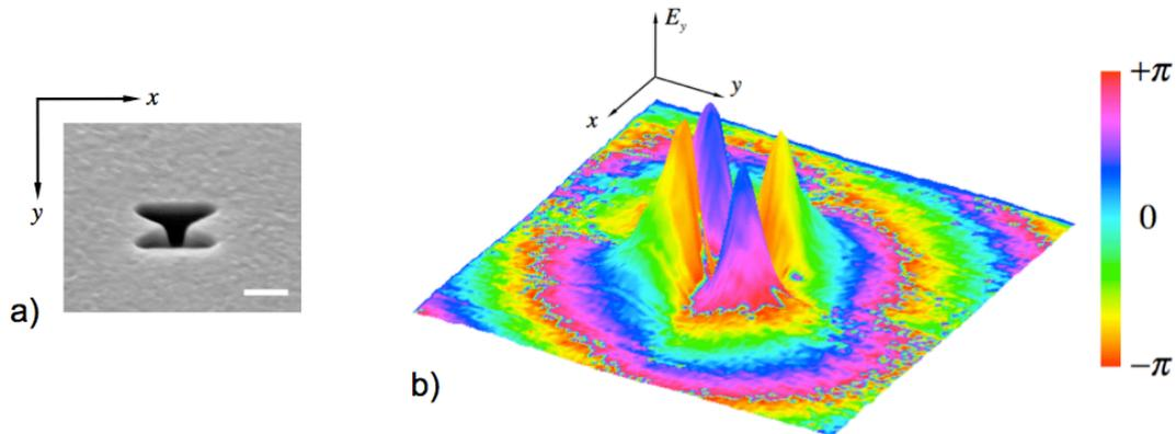
**Figure 1:** a) SEM picture of the bowtie nanoaperture optical antenna. Scale bar is 200nm. b) Experimental mapping giving four lobes pattern for the field component perpendicular to the gap mode, amplitude (z axis) and phase (map color). Scan size is  $2\mu\text{m} \times 2\mu\text{m}$ .
