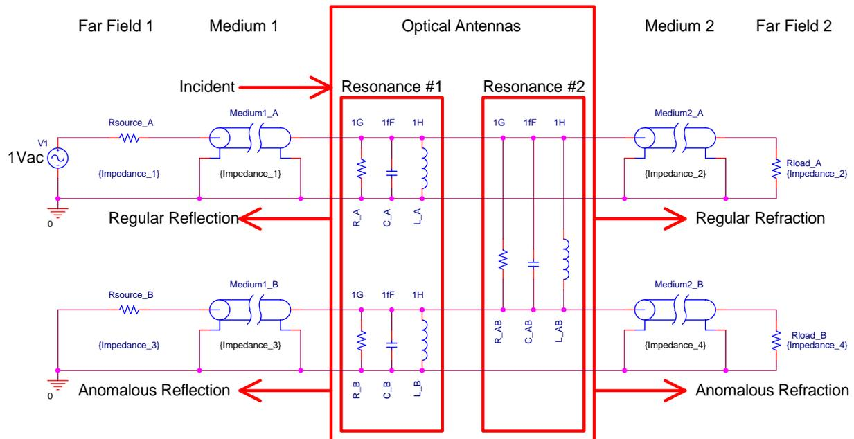
**Fig. 1:** Equivalent circuit, with coexisting lumped and distributed impedances, of the metainterface that generalizes reflection and Snell's laws [1]. The figure is a snapshot from Spice, the well-known electronic simulator, which has been used to simulate the Fresnel coefficients (results are not shown here, but will be discussed in the presentation).
