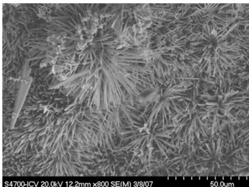
Fig 1: MEB micrograph of Mn-doped ZnO fibres.
