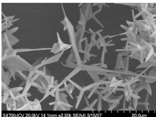
Fig 2: MEB micrograph of pure ZnO tetrapod
