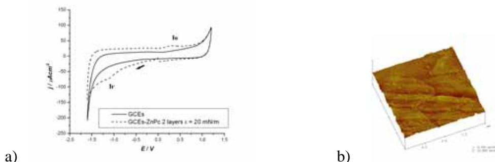
Figure 1. a) Voltammogram, and b) AFM image, of a ZnPc LB film at  $\Pi=20$  mN/m.
