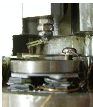
**Fig 1.** Tuning-fork low-temperature nanotribometer.
