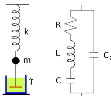
**Fig 2.** (Left) Mechanical model,  $m$  is effective mass of the fork's arms,  $k$  is static spring constant and  $g$  is the damping rate term. (Right) Electrical model. Butterworth-Van Dyke circuit.
