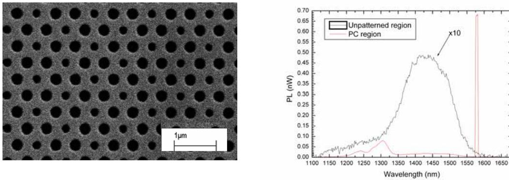
Fig.1. Left panel: SEM micrograph of the fabricated hybrid triangular-graphite structure. Right: Room-temperature photoluminescence spectra at of the PC structure (red line) and of the unpatterned sample (black line).
