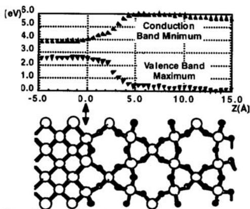
Fig. 1. Non-abrupt band-gap transition at the Si-SiO<sub>2</sub> interface (top), corresponding to the *ab-initio* simulated atomic structure of the interface (bottom), from Kaneta et al. [2].
