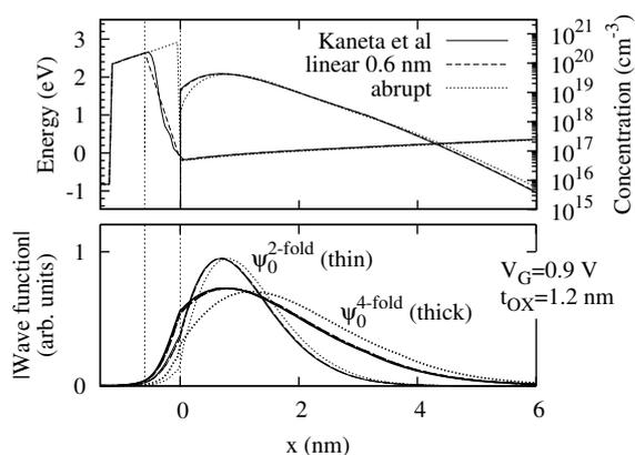
Fig. 2. Conduction band profile and electron density (upper) for three different band profiles at the interface - abrupt, linearly graded, and the band profile extracted from Fig. 1. Normalised wave functions (modulus) corresponding to the lowest sub-bands in the 2- and 4-fold valleys (lower).
