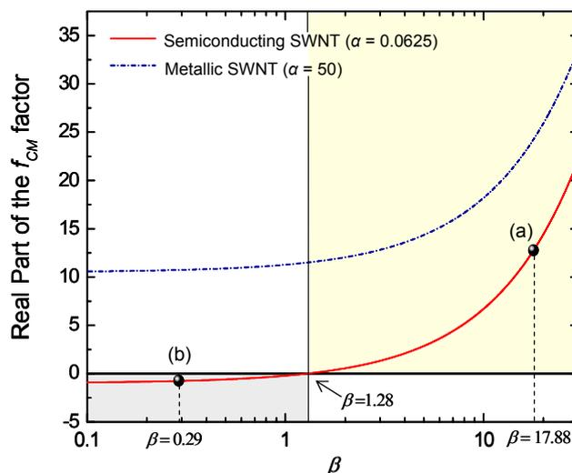
Figure 1 Theoretical plot showing the variation in the real part of the Clausius-Mossotti ( $f_{CM}$ ) factor as a function of two parameters,  $\alpha = \epsilon_p/\epsilon_m$  and  $\beta = K_p/K_m$ . The real part of  $f_{CM}$  was zero at  $\beta = 1.28$  (a)  $\beta = 17.88$  was calculated for the SDS suspended SWNT ( $\zeta = 50$  mV). (b)  $\beta = 0.29$  was calculated for the CTADS suspended SWNT ( $\zeta = 5$  mV). [5]
