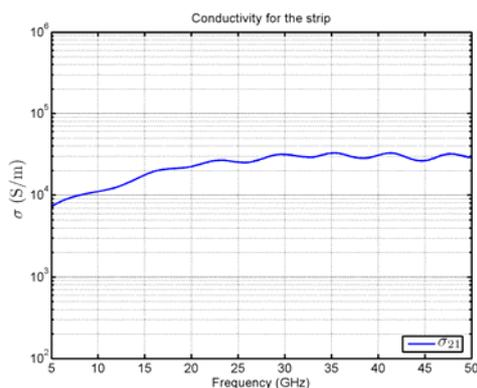
Figure 2. Preliminary results on the conductivity of a CNT bucky paper strip measured in a microstrip transmission line. It can be observed how the value of the conductivity is in the order of  $10^4$  S/m
