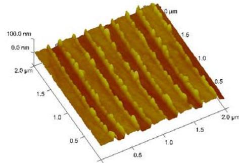
Figure 4: AFM nanograting structures
