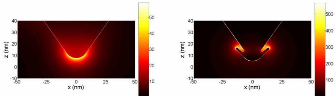
**Fig. 1:** (Left) Near-field distribution around a silver rounded tip with a radius of curvature  $R=10\text{nm}$  for a polarized planewave coming from the left hand side. (Right) Near-field distribution around a nanospear shaped tip, with the same overall radius of curvature. An amplitude field enhancement larger than 500 is observed around the arms of the nanospear
