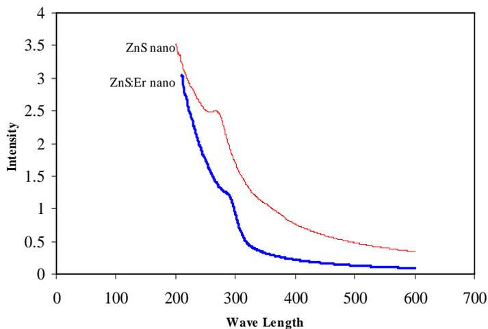
**Fig.1** Absorption spectra for doped and undoped ZnS
