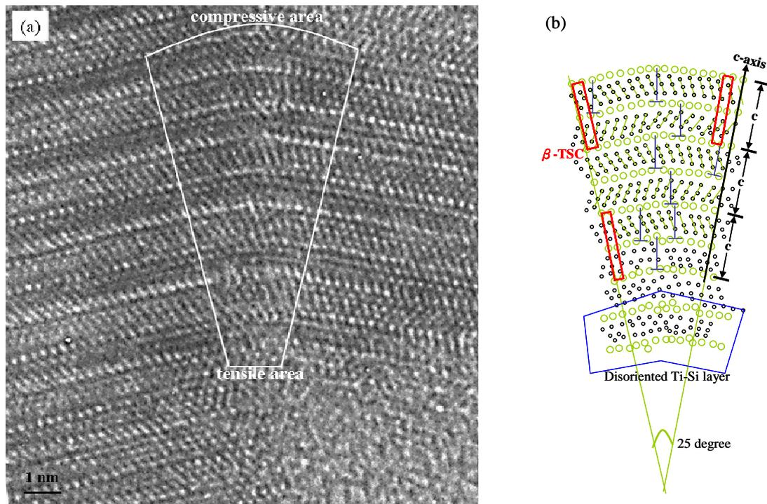
Figure 1. (a) HRTEM image of bending area. (b) Compared atomic position recorded from fan-shaped frame in (a). Green and black circle represents Si and Ti position, respectively.
