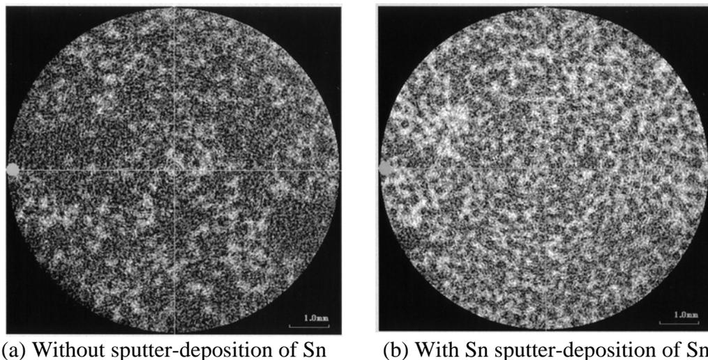
**Fig. 3.** X-ray C.T. images for porous structures of the sintered porous compacts with the porosity 80% obtained from aluminum powder without the tin sputter-deposition(a), and with the tin sputter-deposition(b).
