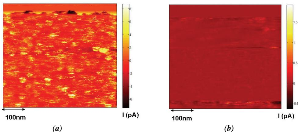
Figure 2. Current maps measured at constant gate voltage of 4.5V in vacuum (a) and 5.8V in air (b) ambient in SiO<sub>2</sub> samples. Measurements in vacuum show better results.
