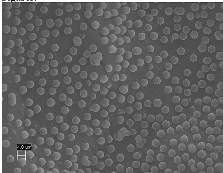
Fig. 1. Scanning electron microscopy image of PS-VBC-DVB microspheres without nanoparticle loading.
