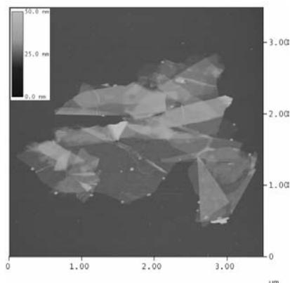
**Fig. 1.** AFM image of a few-layer graphite plate.
