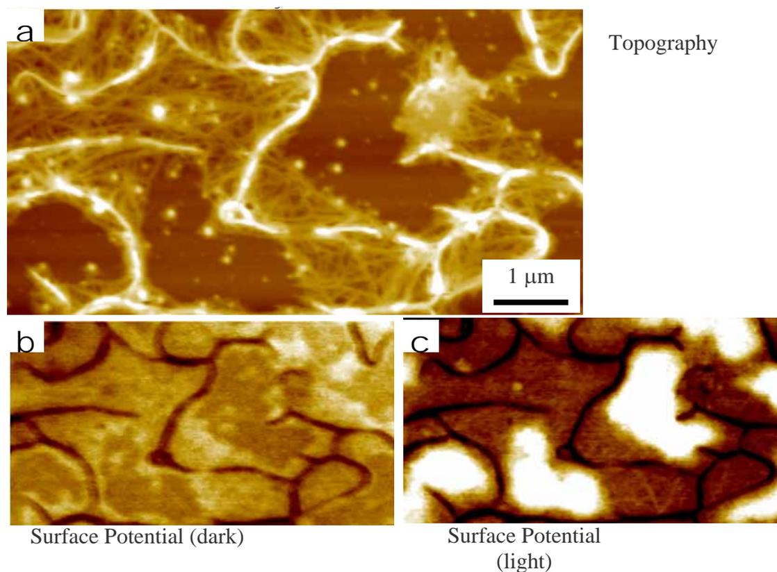
**Fig. 2** a) SFM topography image of an ultra-thin blend of P-PDI and polythiophene deposited on silicon. b) Surface potential image of the same area as in a), with no illumination and c) under white light ( $\sim 60 \text{ mW cm}^{-2}$ ) illumination. Z range: a) 32 nm, b) 120 mV and c) 120 mV.
