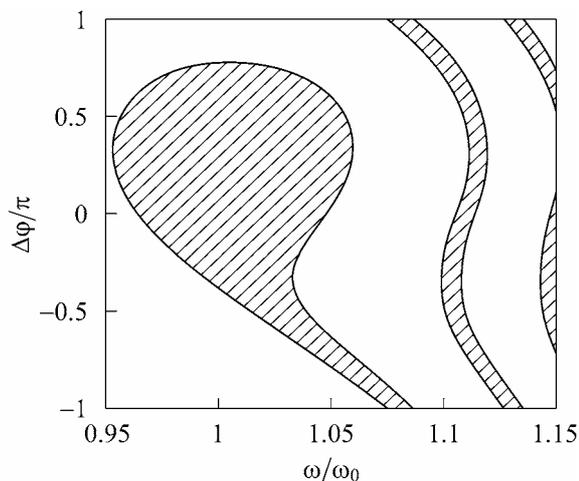
Fig. 3. Start phase shift  $\Delta\phi$  and the frequency ratio  $\omega/\omega_0$  where the stationary mode is possible in the case of system with  $Q = 100$  and control force amplitude  $F_0 = 2F_0^{cr}$  are hatched
