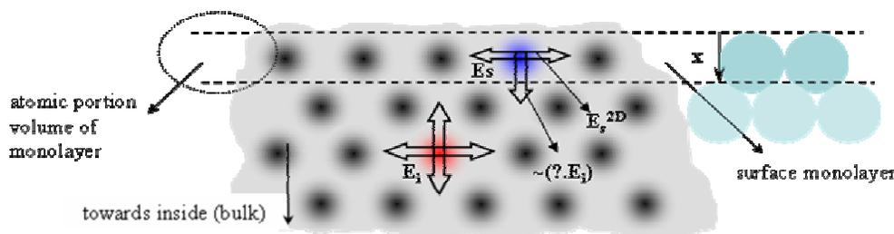
Fig. 1 Schematic representation of bulk and surface of metallic nano-particles considering different binding energies.
