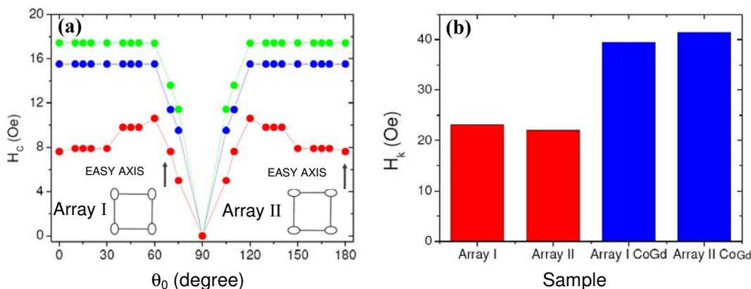
Fig. 3: (a) Angular dependence of the coercivity for magneto-optical transverse Kerr effect hysteresis loops. Red circles, Array I with empty holes; blue circles, Array I with  $\text{Co}_x\text{Gd}_{1-x}$  filled holes; green circles, Array II with  $\text{Co}_x\text{Gd}_{1-x}$  filled holes (b) Anisotropy field values for: Arrays I and II with empty holes (red); Arrays I and II with  $\text{Co}_x\text{Gd}_{1-x}$  filled holes (blue).
