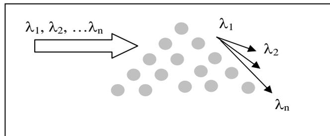
Fig. 1 Schematic diagram of the PBG superprism
