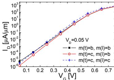
**Fig. 11:** The detail of  $I_D$ - $V_G$  characteristics for the 6 nm gate length, 1.3 nm body DG MOSFET. The effect of systematically replacing bulk values of  $m(t)$  and  $m(l)$  with their confined values is demonstrated.
