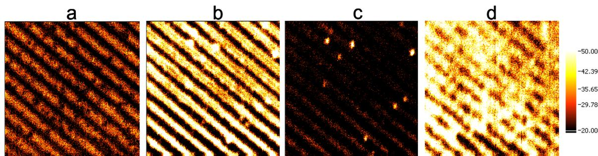
Figure 2. Fluorescence images of  $15 \times 15 \mu\text{m}^2$  areas of a glass substrate with stripes of catechol-based molecules on top after successive exposure of the sample to: (a) air; (b)  $\text{Et}_3\text{N}/\text{N}_2$  flow; (c)  $\text{HCl}/\text{N}_2$  flow; (d)  $\text{HCl}/\text{N}_2$  flow for 5 min. All six images were recorded with the same instrument settings. The fluorescence intensity scale is also equal for all displayed images.
