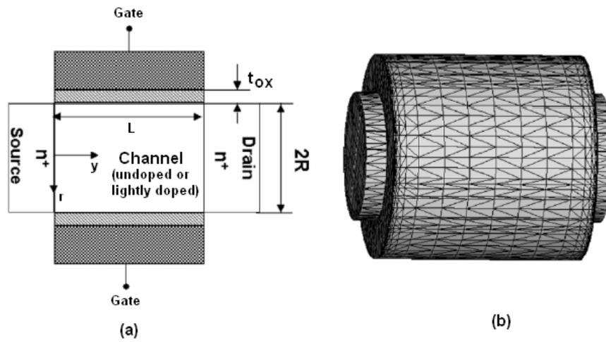
**Fig. 1.** (a) Cross section of the SG-MOSFET. (b) Simulated geometry of the SG-MOSFET using ISE-TCAD<sup>TM</sup>.
