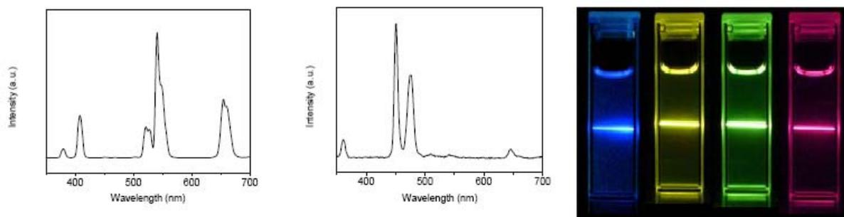
Figure 2 Fluorescence spectra of hexagonal-phase  $\text{NaYF}_4$ : Yb, Er/Tm nanocrystals (left, middle) and photographs showing the upconversion fluorescence from the nanocrystals when irradiated by a 980nm laser (right).
