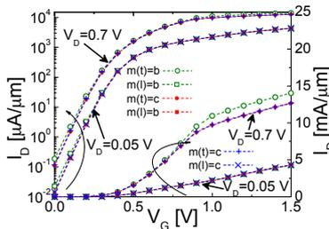
**Fig. 8:**  $I_D$ - $V_G$  characteristics for the 6 nm gate length, 2.6 nm thick body DG MOSFET comparing the effect of confined (c) and bulk (b) Si masses in transversal  $[m(t)]$  and longitudinal  $[m(l)]$  transport directions.
