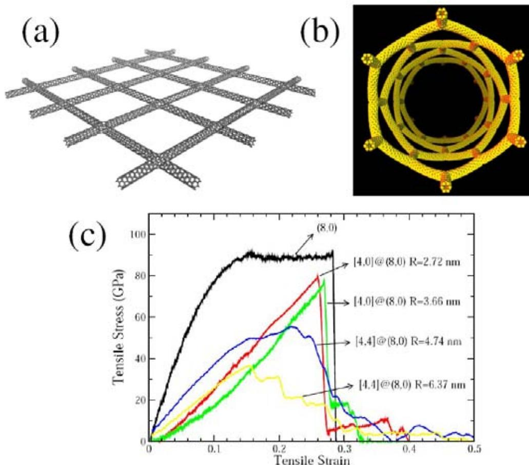
**Figure 1:** (a) Crossbar ordered single walled carbon nanotube network. (b) Configuration of a [6,0]@(6,0) super carbon nanotube. (c) Tensile failure behavior for super carbon nanotubes with different chiralities and radii (R) and for the (8,0) SWCNT at 300 K.
