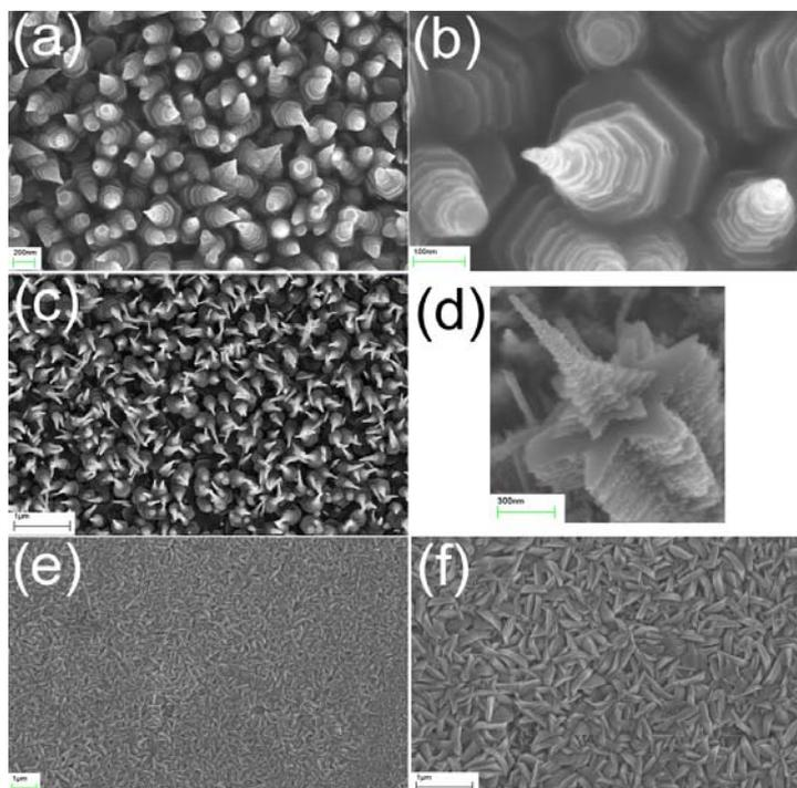
ZnO nanostructures from solution growth methods.
