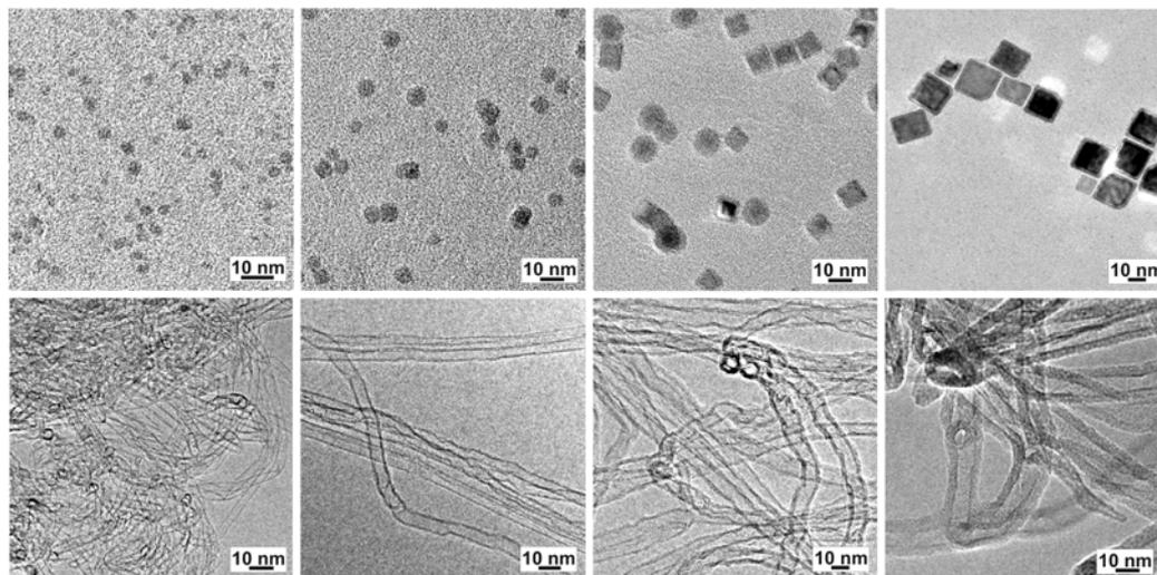
**Figure 2.** Upper panels: TEM images of the starting Fe catalyst particles. Increasing size from left to right. Lower panels, resultant CNT after CVD synthesis on Si/SiO<sub>2</sub>/Al<sub>2</sub>O<sub>3</sub>.
