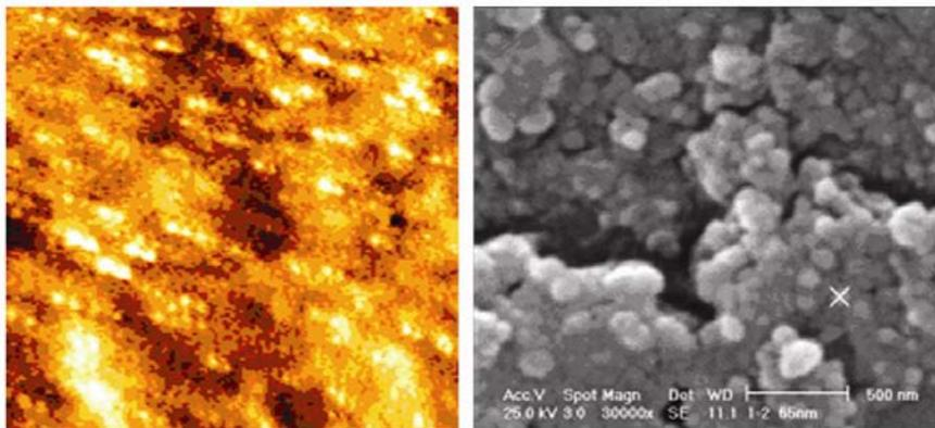
**FIGURE 1. The AFM and SEM images of Gelatin nanoparticles at optimum condition**
