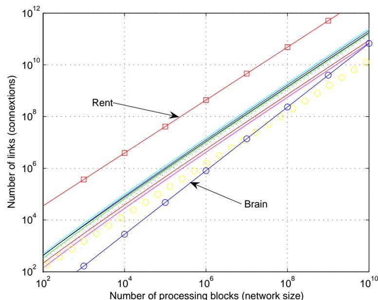
Figure 1. The number of processing blocks (network size) versus the number of connections (links).
