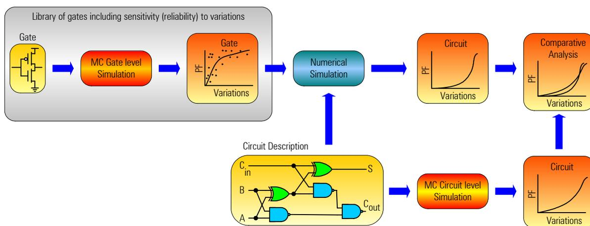
**Figure 1.** Hybrid MC-PTM Simulation Flowchart.
