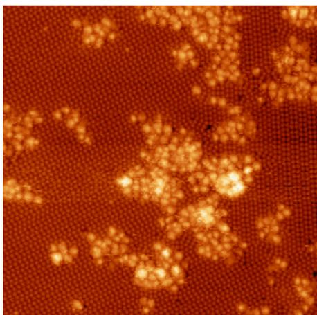
**Fig. 1:** STM image ( $50 \times 50 \text{ nm}^2$ ) showing disordered molecular islands of PTCDA as well as clean substrate areas presenting the Ge(111)-c(2x8) reconstruction. Tunneling parameters:  $V_s = +1.5 \text{ V}$ ;  $I = 85 \text{ pA}$ .
