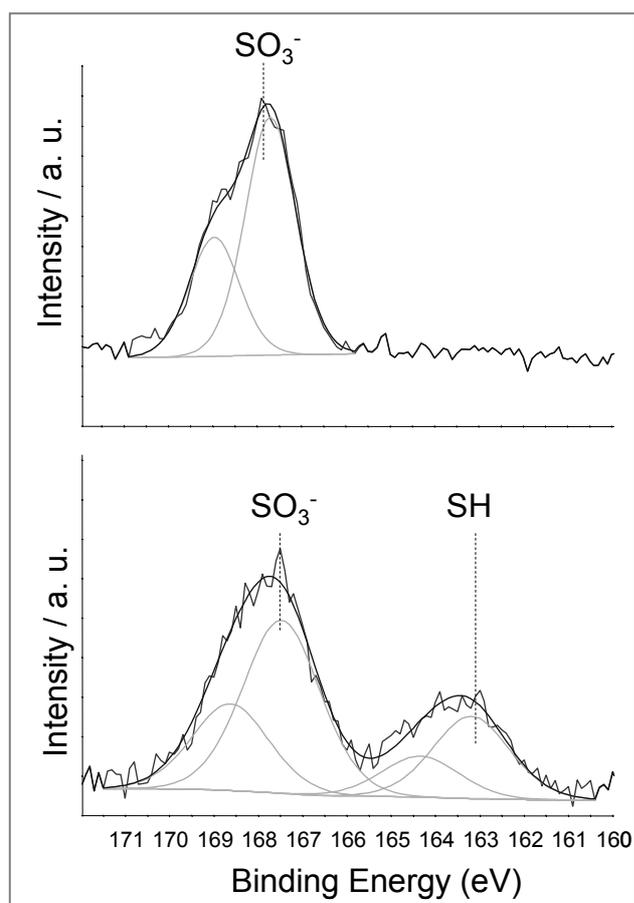
Figure 1.  $S_{2p}$  XP spectra relevant to the pristine (*upper panel*) and etched (*lower panel*, etch time = 160 s) chitosan nanoparticles. Doublet attribution is reported as a label of the  $S_{2p_{3/2}}$  peak.
