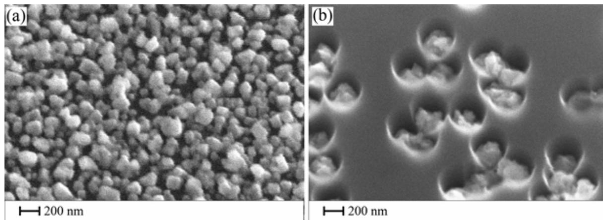
Figure 1. SEM patterns of PbSe electrodeposited at  $E = -0.43$  V from 0.1 M HNO<sub>3</sub> + 50 mM Pb(NO<sub>3</sub>)<sub>2</sub> + 1 mM SeO<sub>2</sub> solution onto Si wafer (a) and into porous SiO<sub>2</sub>/Si template (b).
