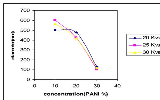
Fig.8. diameter vs. PANi concentration as the voltage increases.
