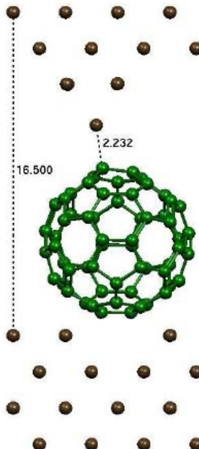
**Fig. 1:** Side view of the  $C_{60}$ -Cu(100) supercell used in the transport calculations.
