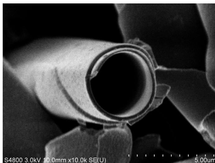
Figure 2. SEM image of tubular  $ZrO_2$  structures.
