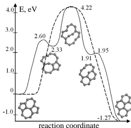
Fig 2.The modified Stone-Wales rearrangement of defects [3]. The solid line corresponds to the one-step process. The dashed line corresponds to the multistep process.
