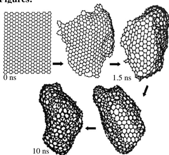
Fig.1. Evolution of a graphite sheet at 3500K.
