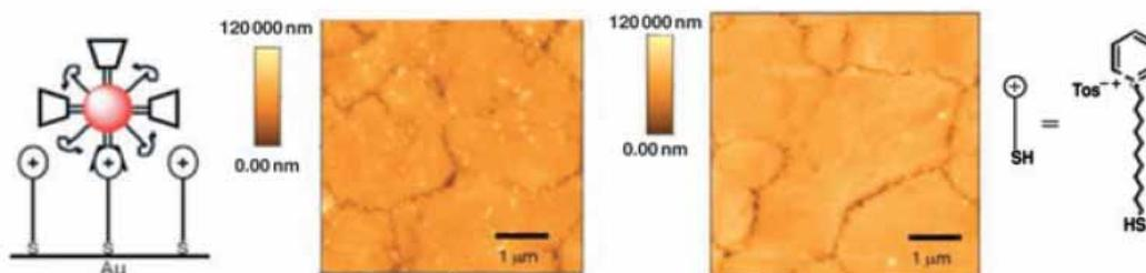
Specific binding of the calixarene-modified gold nanoparticles, from aqueous solution to a self-assembled monolayer (SAM) of the pyridinium salt on a gold surface shown by AFM (left). The control experiments (right) show the nonspecific attachment of only very few particles to the SAMs.
