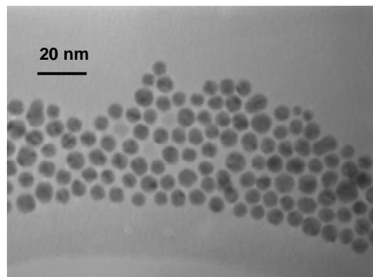
Fig. 1. TEM picture of Fe<sub>3</sub>O<sub>4</sub>@Au NPs.
