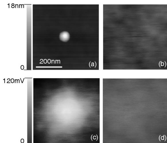
**Fig.3** Topographic image (a) and corresponding surface potential images of an isolated Si dot with a Ge core with a total dot height of ~18nm measured by AFM/Kelvin probe mode before (b) and after injected (c) at +3V, and after electron emission at -1V from the charged Si dot in the tapping mode (d).
