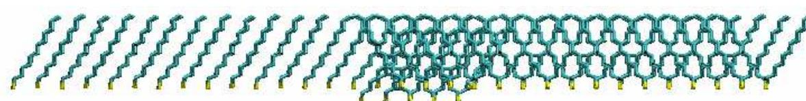
Figure 3: Side view of dodecanethiol SAM incorporating a domain boundary on the right hand side and a depression in the centre (hydrogens are omitted for clarity).
