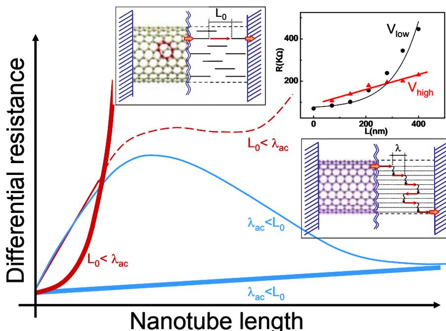
**Figure 1.** This figure summarizes the different electron transport regimes for SWCNTs with and without defects as a function of the bias voltage and length. The thick lines apply to the low bias voltage. The thin lines apply for the high bias voltage. The blue curves are for defect-free SWCNTs (lower inset) and the red ones for defected SWCNTs (upper left inset). The upper right inset shows experimental  $R(L)$  at low and high bias voltages for a defected SWCNT.
