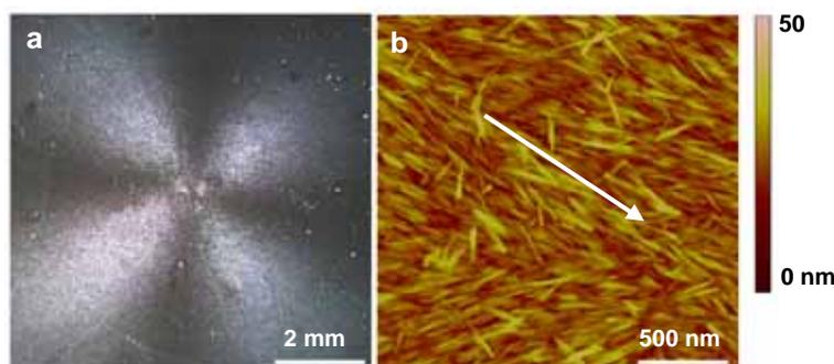
The orientation of cellulose nanocrystals can be seen on many length scales. a) Polarized-light microscopy image of LbL films of (PAH/cellulose)<sub>10</sub> b) tapping mode AFM height image of the same film.
