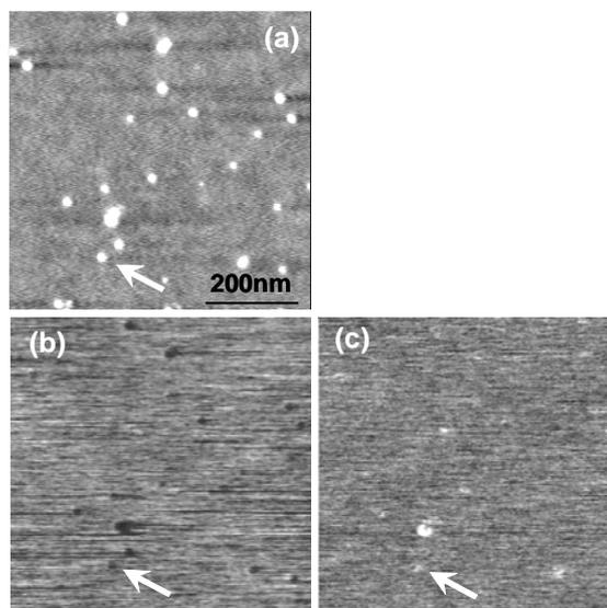
Fig. 2. (a) Topographic and (b), (c) potential image of Co-BND on  $\text{SiO}_2$  surface. Topography was observed tapping mode AFM. Charge injection was carried out at (b)  $V_{\text{sub}} = -2.0$  V and (c)  $V_{\text{sub}} = +2.0$  V, respectively. Corresponding position of BND is indicated by arrow.
