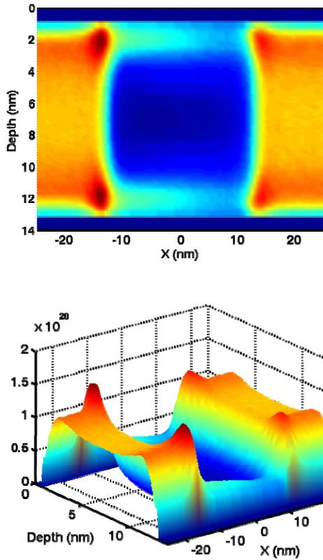
**Figure 1.-** Electron density distribution in a DGSOI transistor
