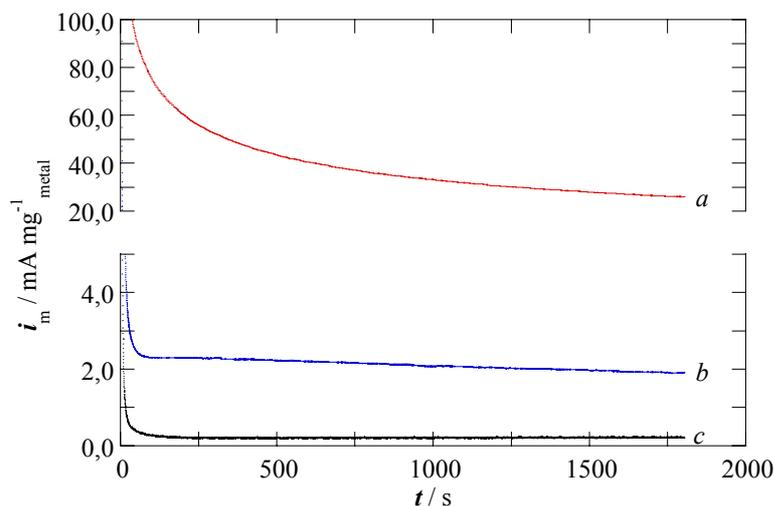
Fig. 3. Chronoamperometric curves of methanol oxidation on DMFC anodes catalyzed by: (a) PtRu/CMK3-Nc0.5, (b) Pt/CMK3-Nd0.5, and (c) Pt/CMK3-Nc2h in 2.0 M  $\text{CH}_3\text{OH}$  + 0.50 M  $\text{H}_2\text{SO}_4$ .  $T = 60^\circ\text{C}$ .  $v_b = 20 \text{ mV s}^{-1}$ .
