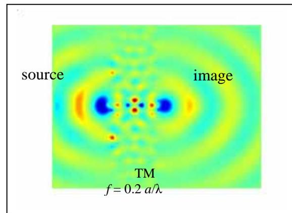
Fig.4 Snapshot of the (TM)  $E_z$
