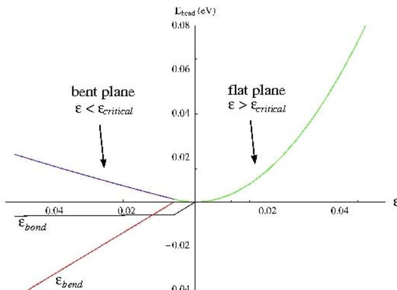
**Figures:** The formation energy of a graphite plane when compressed ( $\varepsilon < 0$ ) or expanded ( $\varepsilon > 0$ ). The green and blue curves represent the formation energies when the strain  $\varepsilon$  is above or under the critical strain  $\varepsilon_{critical}$ , respectively. The red line represents the strain component due to the bending, while the black line represents the strain component in-plane compression.
