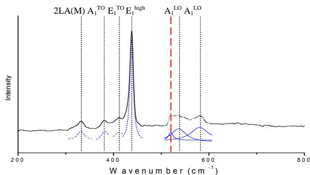
Fig3. Room temperature Raman spectra of Mn:ZnO carpet type fibres. The black line corresponds to the experimental spectra and the blue lines to the Lorentz fitting.
