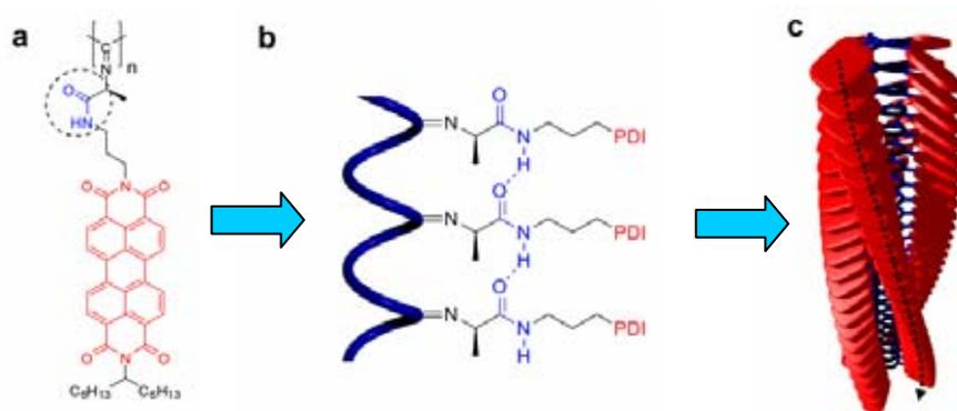
Fig.1 a) Chemical structure of a multi-chromophoric array based on poly(isocyanide) units functionalized with perylene (P-PDI); The amide unit responsible for the hydrogen bonding that stabilizes the helical structure is encircled. b) due to hydrogen bonding, the polymeric chain adopts a coiled structure. c) Cartoon showing the complete helical structure of the P-PDI. The dashed arrow indicates one of the four stacks of PDI units present along the central polyisocyanide backbone.
