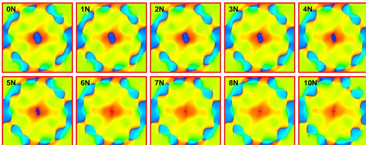
Fig. 3. The  $H_x$  phase component ( $O_z$  section at the end of the FO) for elongating (loading) forces  $F$  in the range 0N to 10N. A “blue opening” is clearly visible in the center at 0N (surrounded in red), but it is quickly fading (see top row), while completely vanishing (disappearing) at 6N.
