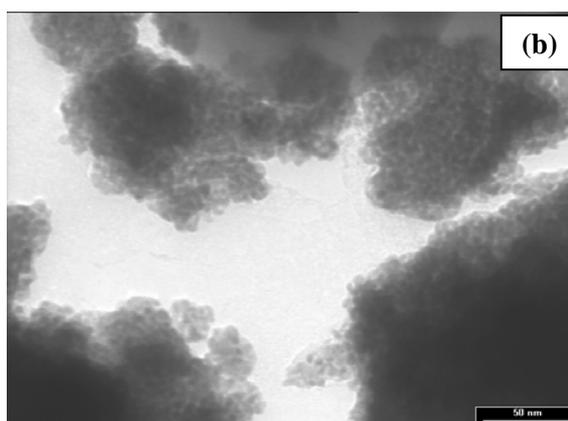
Figure 4. Electronic transmission microscopy of powder "S" (a) and "ZS" (b) thermal treated at 1000<sup>0</sup>C/2h
