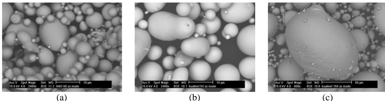
Figure 1.- SEM microstructure of the as-received powders (a) AW2-08 and KUALMET (b) < 53 μm (c) < 150 μm.
