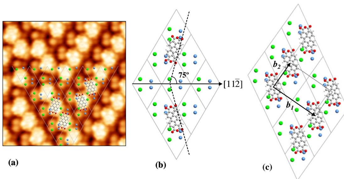
**Figure 2** (a) High resolution STM image shows that within each substrate domain, there are two preferential orientations of the molecule related by mirror symmetry relative to the  $[11\bar{2}]$  substrate direction (10nm $\times$ 10nm,  $V=+2.0V$ ,  $I=0.1nA$ ). (b, c) Proposed structural models indicate the molecular adsorption geometry and the PTCDA commensurate  $(4\sqrt{3}\times 2\sqrt{3})R30^\circ$  structure on the Si(111)- $2\sqrt{3}\times 2\sqrt{3}$ -Sn surface, respectively.
