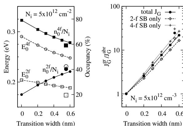
Fig. 5. Sub-band energy and occupancy (left), and direct tunnelling current (right) dependence on transition width for a constant inversion charge,  $N_i$ . The non-connected points correspond to the band-gap transition profile from Fig. 1. These results are independent of the simulated oxide thickness.
