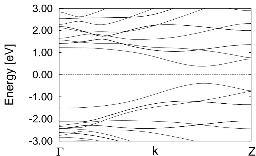
FIG. 2: Band structure of a (6,6) CBNNT showing the opening of a gap, where the CNT analog would be metallic. The dashed line corresponds to the Fermi level.
