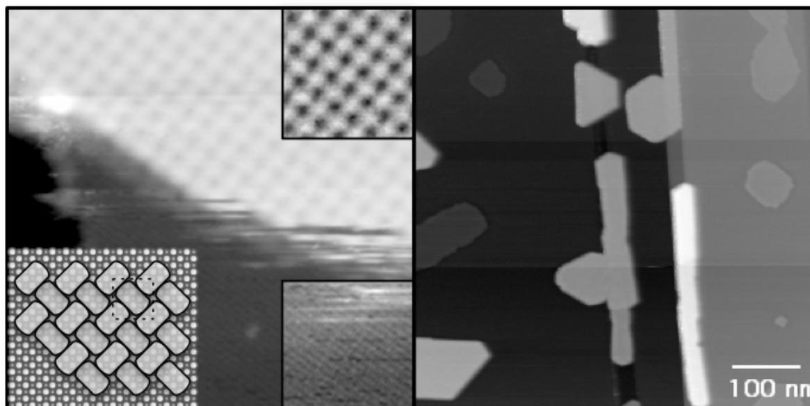
**Fig. 2:** High resolution nc-AFM on PTCDA overlayer on NaCl with insets adjusted for better contrast (left) used to determine the strained  $c3 \times 3$  epitaxy (lower left inset). Overview image of co-existing monolayer and multilayer islands at 0.8ML coverage (right)
