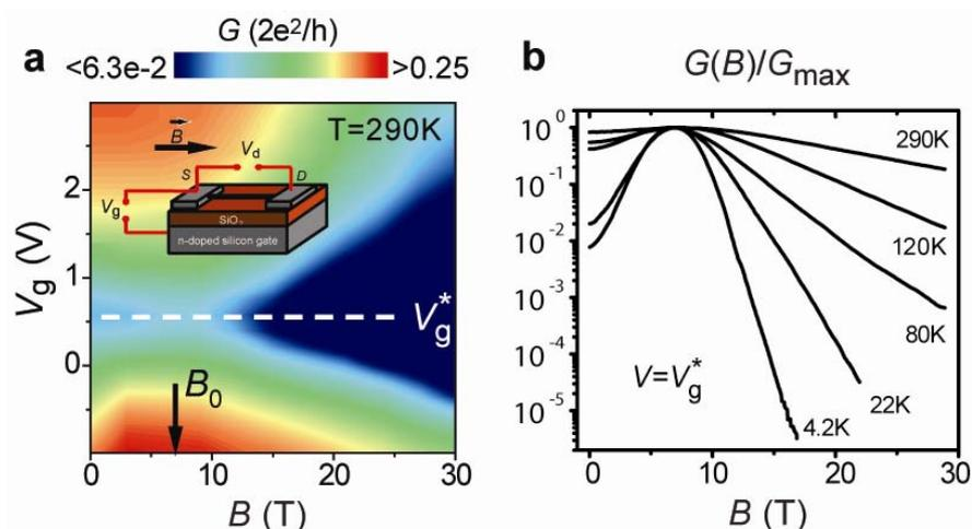
**Figure 1.** Magnetically induced field effect in carbon nanotube based devices. (a) Plot of the sample 1 conductance versus the gate voltage and the axial magnetic field. A dark arrow indicates the value of  $B_0$ , where the gap  $\epsilon_g(B)$  has a minimum. (b) Off-state magnetoconductance of sample 1. At  $B > 10$  T the  $G(B)$  curves appear as straight lines in the log-vs-linear scale
