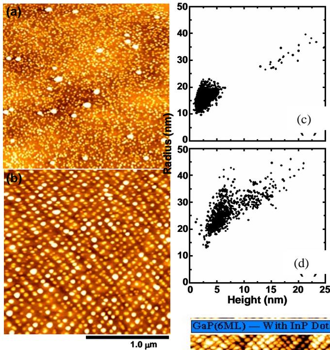
Fig.1 – AFM images and dot size distribution for InAs dots grown on (a,c) GaAs and (b,d) the InP template (GaAs/InP/InGaP/GaAs); (bottom) HRTEM image showing the vertical correlation between InAs and InP dots.
