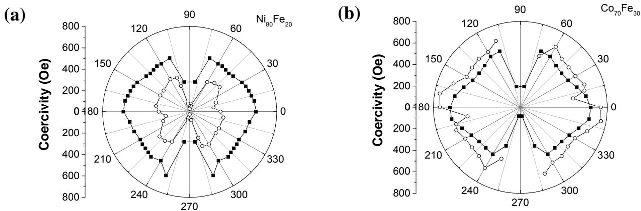
Figure 3. Coercivity angular dependence of  $\text{Ni}_{80}\text{Fe}_{20}$  (a) and  $\text{Co}_{70}\text{Fe}_{30}$  (b). In each sample, the open circles correspond to an square symmetry and the filled squares to an hexagonal symmetry.
