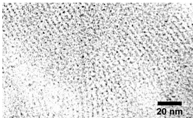
**Fig. 1:** TEM image showing maltose-protected gold nanoparticles perfectly aligned. The neoglycoconjugate forms micelles with a tubular shape and gold cores are found encapsulated in the organic material.
