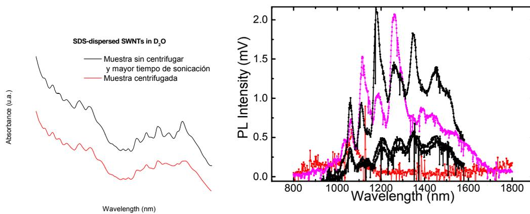
Fig.1. Left: Spectra of the absorption of the SWCNTs diluted in D<sub>2</sub>O for different sonication times. Right: Room temperature photoluminescence spectra showing the emission of the SWCNTS in D<sub>2</sub>O.
