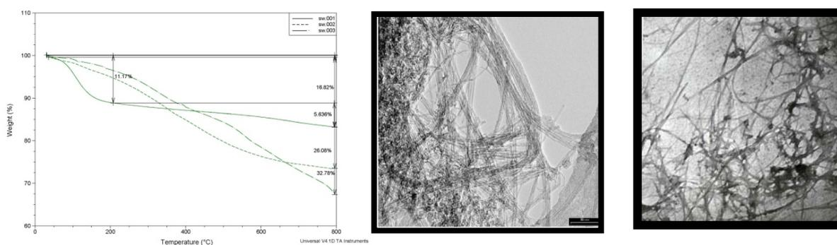
**Figure 1.** (left) TGA of **1** (—), **2**(...) and **3** (-.-), (middle) TEM image of **1**, (right) TEM image of **3**.
