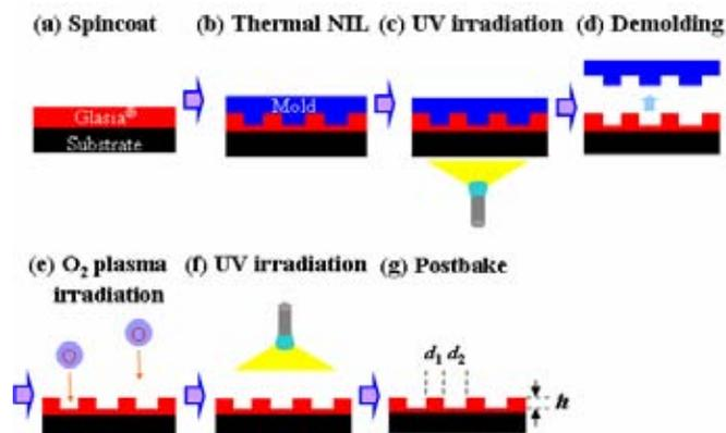
Fig. 1: Our single-step fabrication of a wave plate using inorganic-organic hybrid glass with nanoimprint lithography. (a) spin coating and prebaking, (b) low-temperature nanoimprint, (c) UV irradiation through a SiO<sub>2</sub> substrate, (d) Demolding of Si mold, (e) O<sub>2</sub> plasma treatment to oxidize and harden the patterned surface, (f) UV irradiation from the patterned surface side, and (g) postbake to further harden the material.
