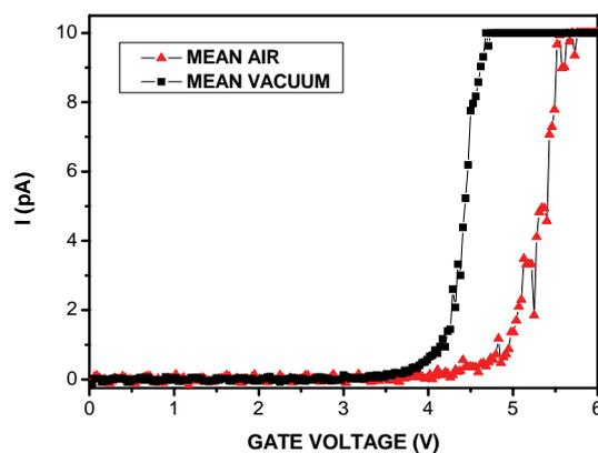
Figure 1. Average of several IV characteristics of a 2nm SiO<sub>2</sub> sample measured in vacuum and air ambient.
