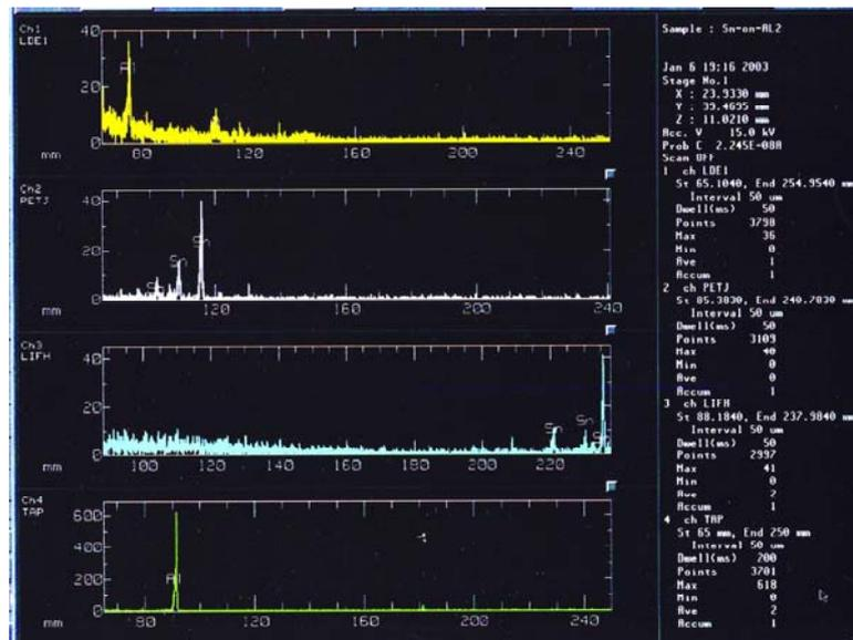
**Fig. 2.** Result of EPMA analysis on the surface of the particles obtained after the sputter-deposition in this study.
