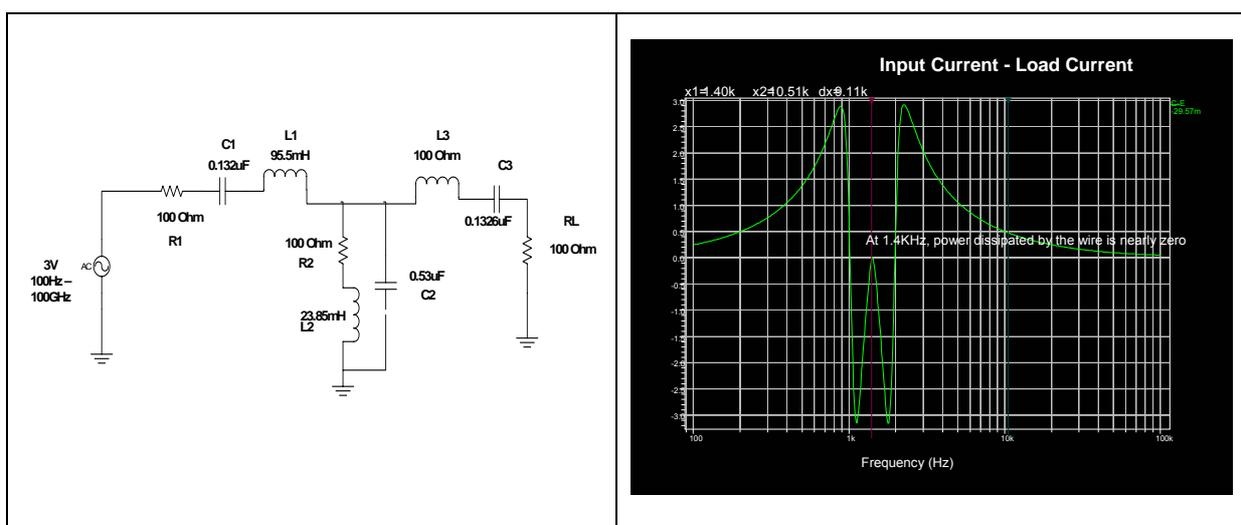
Figure 2.:Schematic for an accurate wire model and plot of difference in currents through Input resistance and RL;
