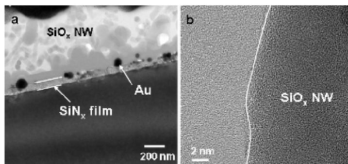
Fig. 2. TEM images of (a) cross section of the sample and (b) high-resolution of a single  $\text{SiO}_x$  NW.
