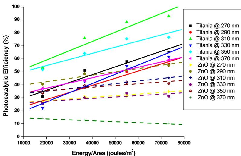
**Fig. 1.** Spectral photocatalytic efficiency of TiO<sub>2</sub> and ZnO nanocomposite films at activation wavelengths (270-370 nm) as a function of incident total optical energy per unit area (incident optical intensity  $\times$  time).
