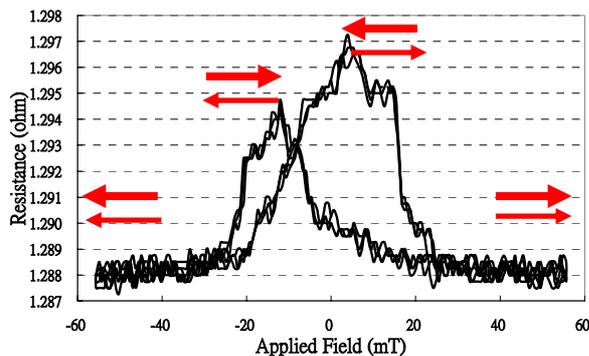
Fig.2 MR curve of the nanopillar
