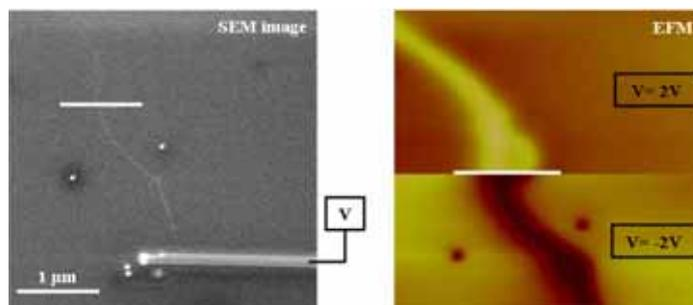
**Figure 2.** Left: SEM Image of a MWCNT contacted by electron beam induced platinum deposition. Right: Electrostatic force microscopy (EFM) image of the MWCNT biased from the contact electrode. The white line shows the correspondence between the EFM and the SEM image. The electrode polarization is reversed ad mid-scan, corresponding to the contrast inversion in the EFM image.
