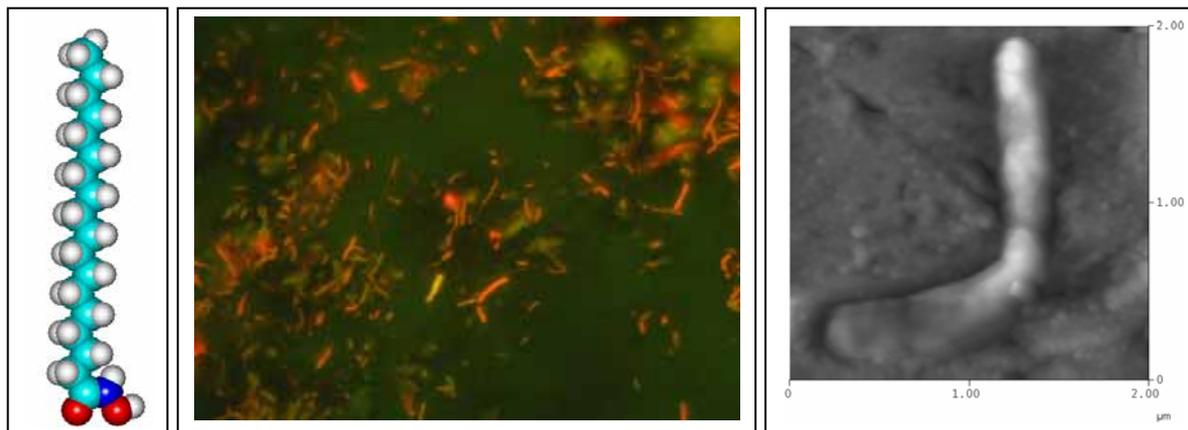
**Figures. Left: Molecule model of the stearyl hydroxamic acid, one of the nanofilm-forming compounds. Middle: Rod-like bacilli on a copper surface imaged under fluorescence microscope after 48 h immersion of the substrate. Right: A dividing bacillus on copper surface (scan area:  $2 \times 2 \mu\text{m}^2$ , z-range: 200 nm)**
