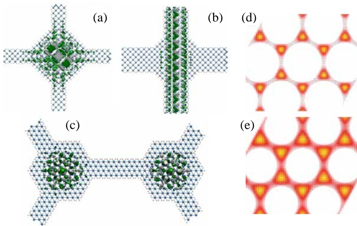
**Figure 2:** Wave-function of the lower state of the conduction band in the case of square and hexagonal arrays of channels in silicon (a,b,c) and GaAs (d,e); showing nanowire (a,c,d) and 2D (b,e) superlattice regimes.
