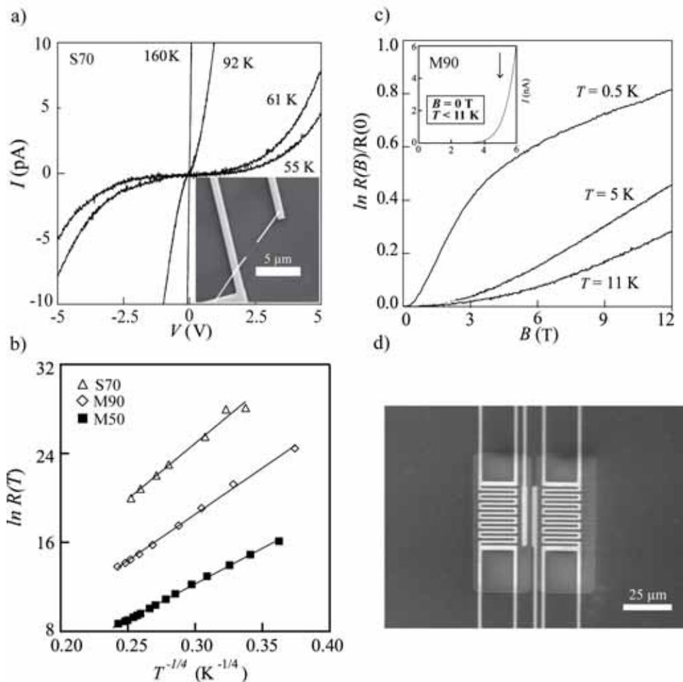
Fig.1 (a)  $I$ - $V$  characteristics of sample S70. (b) VRH plots for samples S70, M90, and M50. The solid lines are fits to the data. (c) Variation of  $\ln[R(B)/R(0)]$  with  $B$  at indicated  $T$ 's for the sample M90. Inset: Below  $T = 11 \text{ K}$  the  $I$ - $V$  curves are indistinguishable. (d) SEM image of the device for thermopower measurements.
