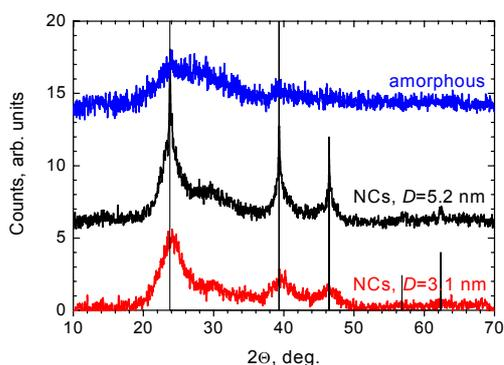
Fig. 1. GIXRD spectra of the CdTe NCs doped  $\text{SiO}_2$  glass films. The peak position of cubic CdTe are shown as vertical lines (from JCPDS database 15-770).
