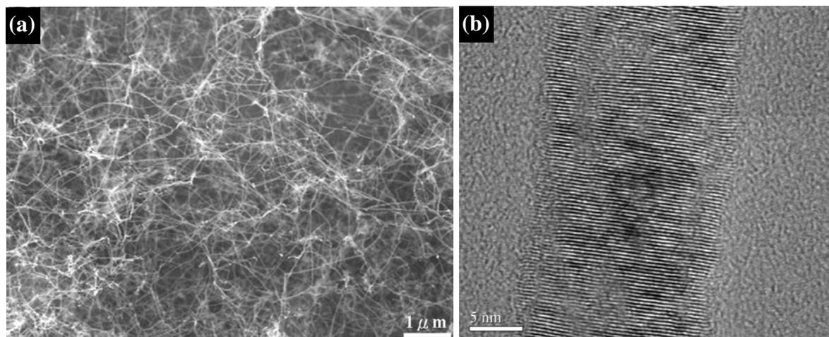
Fig. 1. (a) SEM and (b) HR-TEM image of PGNFs.
