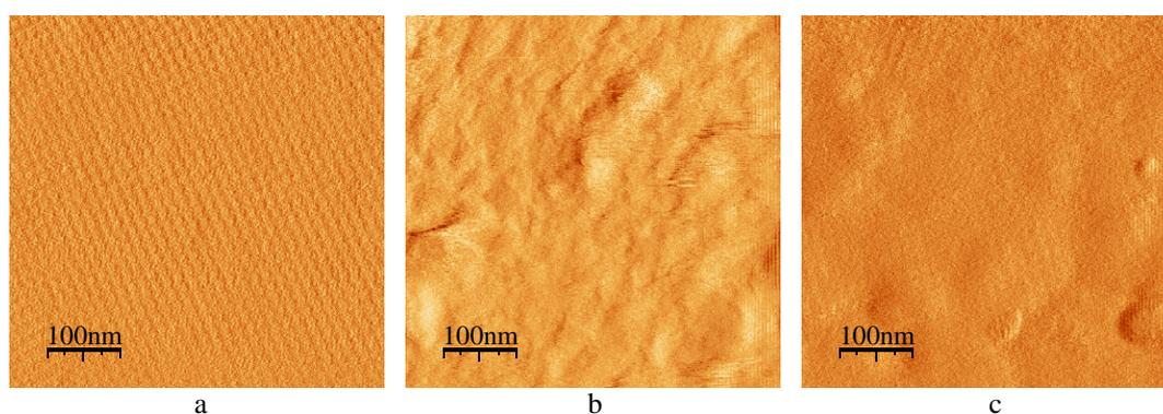
Figure 1. Atomic force microscopy deflection images of S-layers recrystallized on PEM. a) S-layer just as it was formed; b) S-layer treated with EtOH/H<sub>2</sub>O 80/20 (v/v); c) Recovered S-layer after treatment with recrystallization buffer (S-layer protein renaturation).
