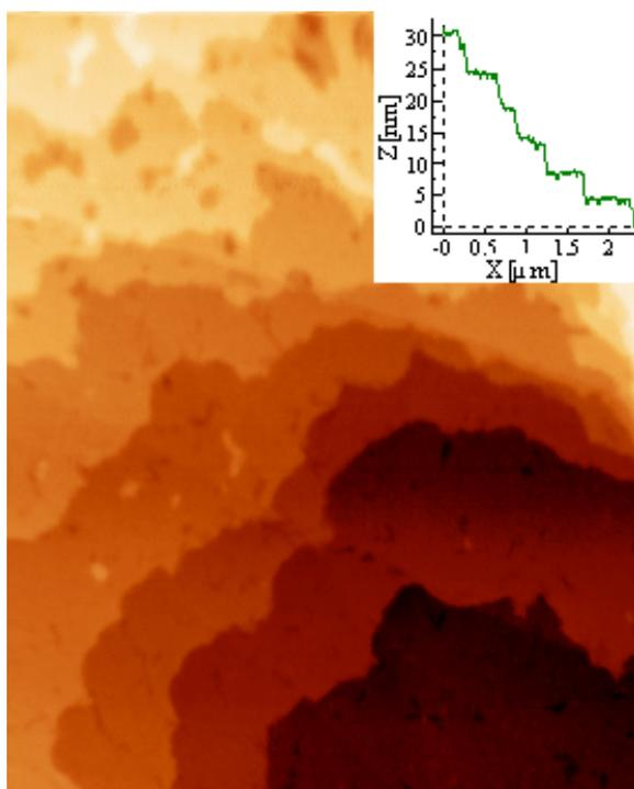
**Fig. 2:** In non-contact AFM mode, more than ten layers of (maltoC<sub>11</sub>S-)<sub>2</sub> molecules were formed on graphite (2.4 x 3 μm<sup>2</sup> AFM image) from the solution containing the glyconanoparticles. The inset shows a profile through eight layers. The height of the graphite terrace visible was used for z-calibration.
