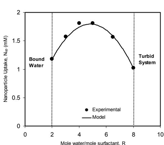
**Figure 1.** Nanoparticle uptake as a function of water to surfactant mole ratio,  $R$ , obtained when mixing a stoichiometric amount of  $\text{CuCl}_2$ -containing microemulsions  $\{[\text{CuCl}_2] = 3.0 \text{ mM}, [\text{AOT}] = 200 \text{ mM}, R = 3.0\}$  with  $\text{NaOH}$  for 3 h at 300 rpm.
