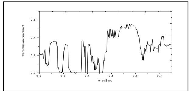
Figure 2 Transmission of the PC with 4 Si/SiO<sub>2</sub>
