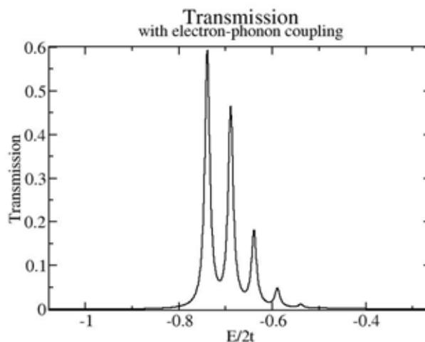
The propagation is performed with the Lanczos algorithm (2), which allows big time steps, rapid convergence, and flexibility in the implementation of the hamiltonian matrix. This last point is extremely important because, as our method permits us to calculate transmissions with an arbitrary number of phonons, we will need to increase the number of phonons until convergence is reached.
