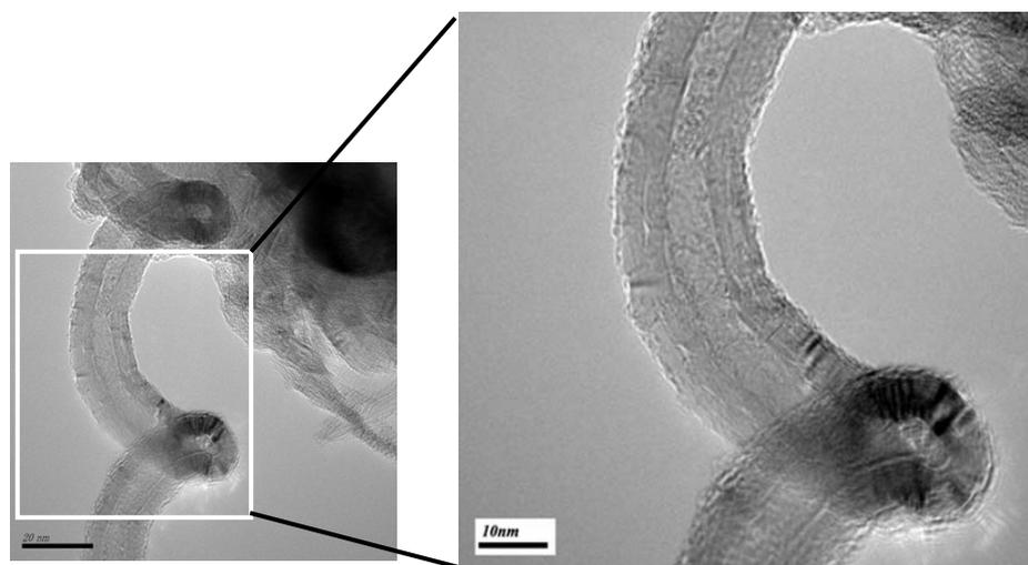
Fig. 3. TEM images of a synthesized CNC
