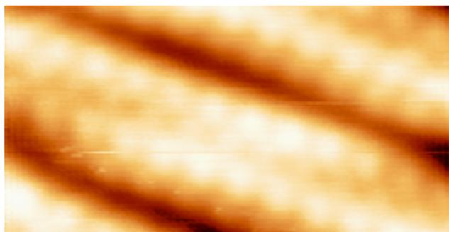
**Left:** Typical STM image of the  $1 \times 2$  reconstruction of the  $\text{TiO}_2(110)$ , showing large chains running continuously along the  $[001]$  surface direction. The total width of the image is  $100 \times 100 \text{ nm}^2$ . **Right:** Typical atomic resolved STM image of the  $1 \times 2$  reconstruction of the  $\text{TiO}_2(110)$ . The total width of the image is  $4 \times 2.7 \text{ nm}^2$ .
