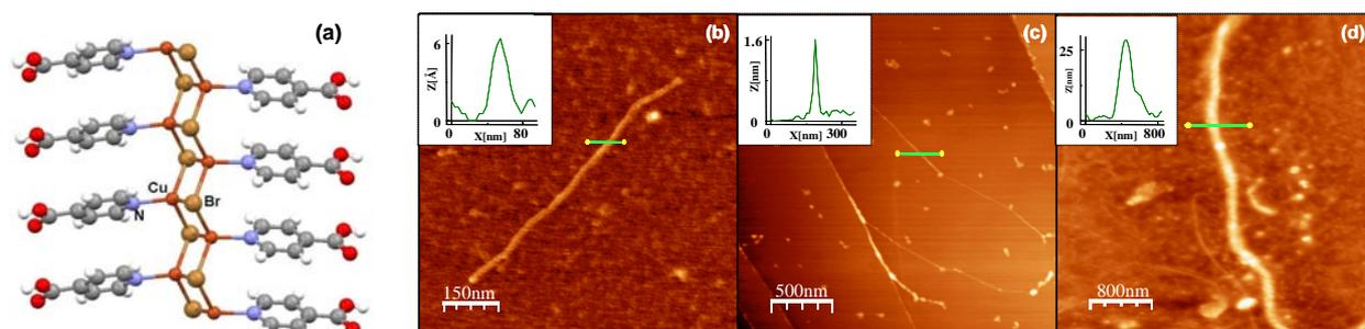
**Figure 1.** (a) Schematic representation of a  $[\text{CuBr}(\text{IN})]_n$  polymer chain. (b) AFM topography image of  $[\text{CuBr}(\text{IN})]_n$  deposited on mica treated with polylysine (b) HOPG (c) and gold (d) surfaces.
