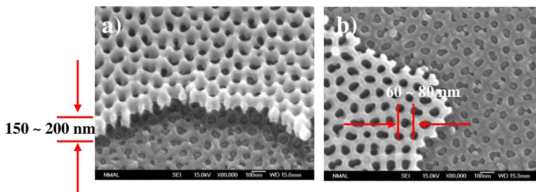
Fig. 1 SEM images of an AAO template(bright part) on a silicon substrate ; a) oblique view, b) top view.
