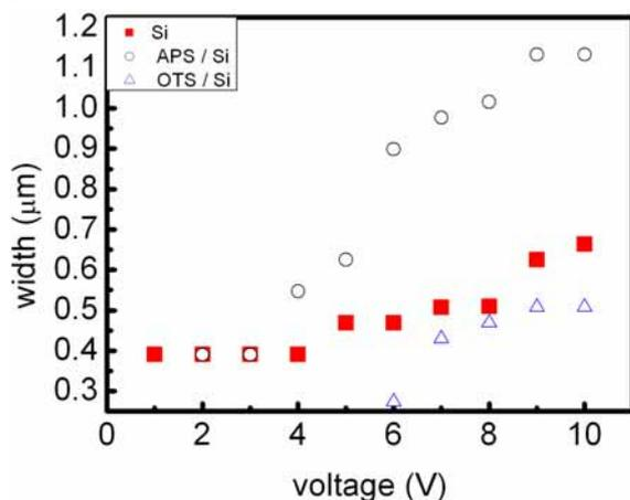
Figure 1: The width of the tip-induced oxidation vs. the applied voltage of the AFM tip under different surface functionalizations.
