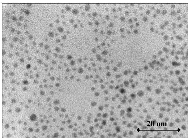
**Figure 1.** TEM micrograph of dodecanethiol-capped Au nanoparticles.
