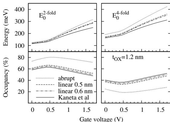
Fig. 3. Sub-band energy and sub-band occupancy (percentage of the total inversion charge density) dependence on gate voltage, for the three different interface band-gap transition profiles, as on Fig. 2, at a given oxide thickness  $t_{OX}$ .
