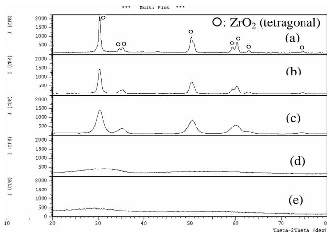
Figure 2. The spectrum of X-ray diffraction obtained on "ZS" powder, for various thermal treatments (a) 1200<sup>0</sup>C/2h; (b) 1100<sup>0</sup>C/2h; (c) 1000<sup>0</sup>C/2h; (d) 700<sup>0</sup>C/2h; (e) as synthesized
