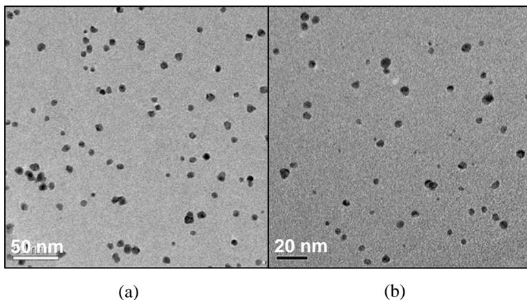
*Fig. 1: Typical TEM image of Pd- (a) and Pd@Cu-PSMNPs (b) prepared by intermatrix synthesis technique.*
