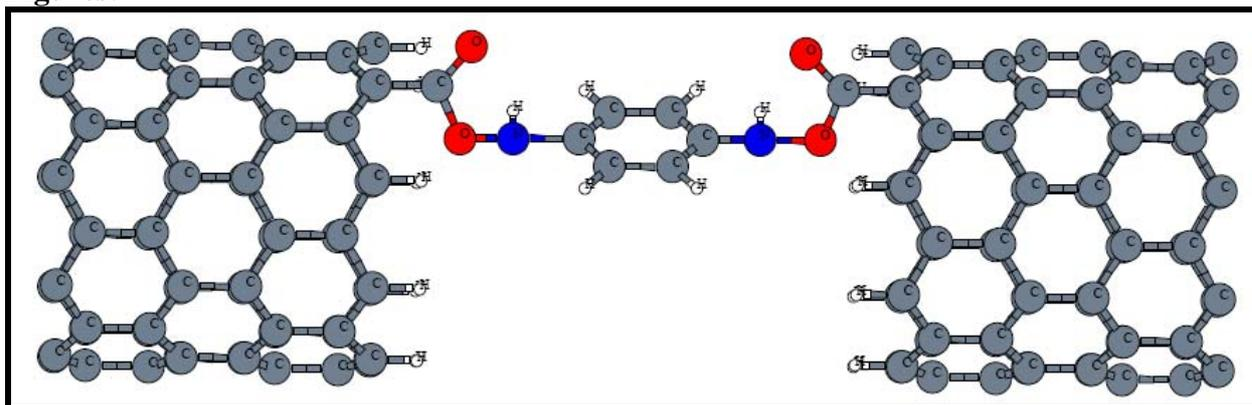
Figure 1 : Benzene molecule coupled to carbon nanotube leads.
