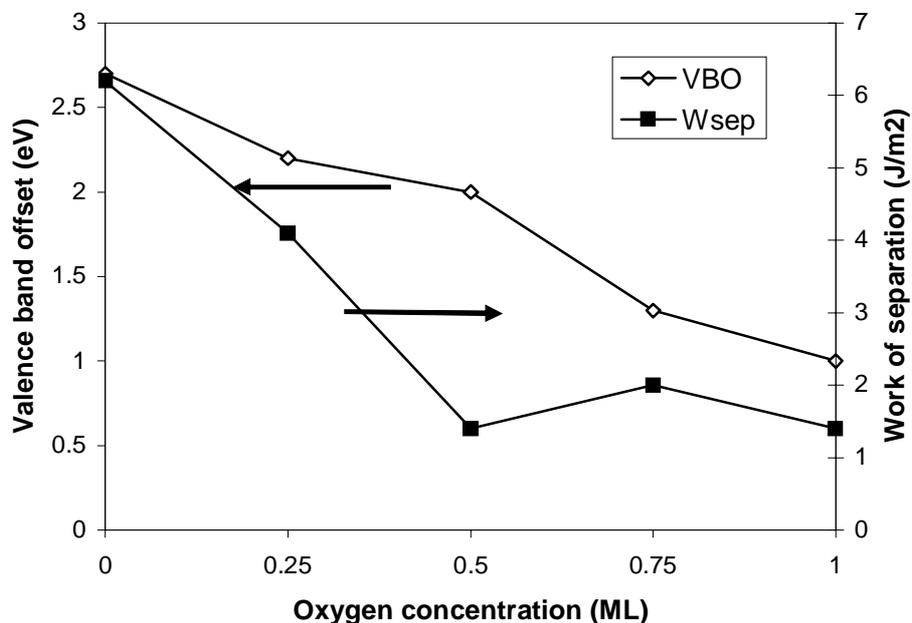
Fig. 1. Calculated valence band offset (VBO) and work of separation ( $W_{sep}$ ) for the Pt/HfO<sub>2</sub> interface as a function of interfacial oxygen concentration.
