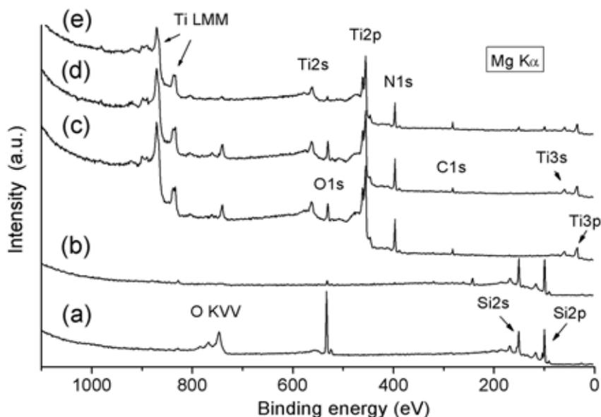
Fig.2. Wide scan XPS spectra of sample surface: (a) substrate before cleaning by ion beam; (b) after cleaning; (c) after titanium sputtering in nitrogen atmosphere; (d) after temperature annealing at 650°C 5 min; (e) after annealing at 750°C 5 min.
