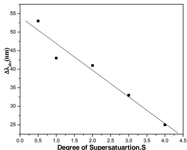
**Figure 2.** A plot of  $\Delta\lambda_{\text{abs}}$  against degree of supersaturation for CdS NCs. (where  $\Delta\lambda_{\text{abs}} = \lambda_{\text{peak}} - \lambda_{\text{onset}}$ )
