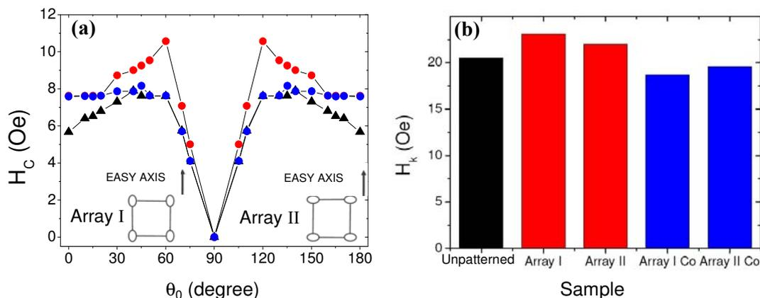
Fig. 2: (a) Angular dependence of the coercivity for magneto-optical transverse Kerr effect hysteresis loops. Black triangles, unpatterned film; red circles, Array I with empty holes; blue circles, Array I with Co filled holes. (b) Anisotropy field values for: unpatterned film (black); Array I and Array II with empty holes (red); Array I and Array II with Co filled holes (blue).
