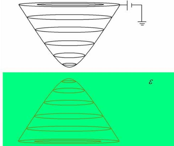
Figure 2. Schematic diagram of the tip made up of charged rings. In the presence of a dielectric material, an image set of charged rings is considered.
