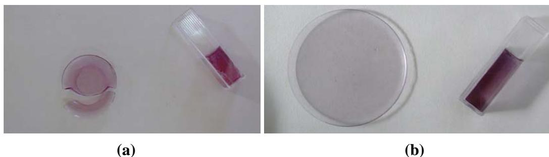
**Figure 2.** Photographs of nanocomposites prepared with (a)  $R=3060$ ; (b)  $R=2470$ .
