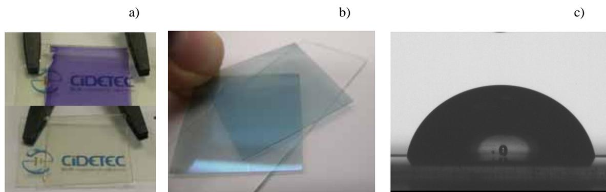
**Figure 1** Nanolayers for optoelectronic devices prepared at CIDETEC. a) Electrochromic device prepared on plastic substrate, b) transparent and conductive layer based on PEDOT on plastic substrate, c) hydrophobic character of PEDOT formulations on plastic substrate.
