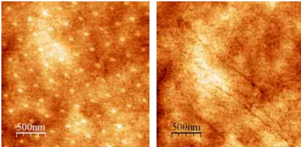
**Fig. 1:** Topography images of an array of W-nanoparticles, measured with normal forces of  $\sim 3$  nN and  $\sim 45$  nN, respectively. Total height 5.2 nm and 4.2 nm, respectively. Scan range 2.5 microns.
