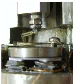
**Fig 1.** Tuning-fork low-temperature nanotribometer.
