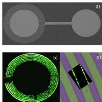
Optical images of: a) Interdigitated bottom-contact device b) Green electroluminescence of HST-LEFT c) magnified contacts and localized light emission
