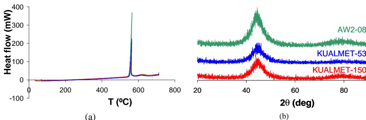
Figure 2.- (a) DSC scans of the three different materials, (b) XRD diffractograms of the three different materials evidencing the amorphous structure of the as-received powders.
