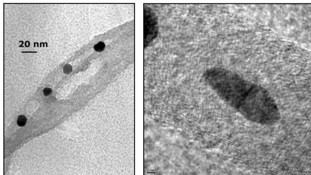
**Figure 1.** TEM and HRTEM images of AuNPs@MWCNTs hybrids obtained by the impregnation method.
