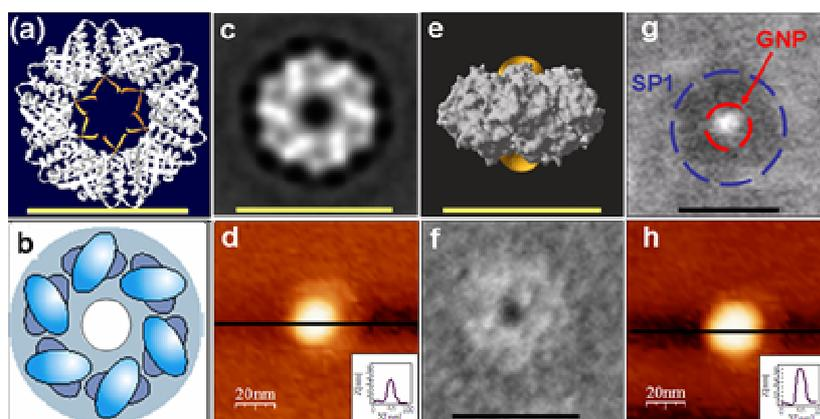
(a) X-ray structure of the SP1, showing the N-termini of the monomers in orange. (b) Scheme of the SP1 dodecamer. (c) Top-view TEM. (d) AFM image of a single dodecamer (inset-cross section). (e) Computer simulation of SP1-GNP in a side view. (f) Top view TEM of SP1-GNP. (g) Top view HAADF-STEM of SP1-GNP. (h) Top view AFM image of single SP1-GNP (inset-cross section). Scale bar 11nm.
