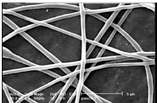
Fig.2. SEM micrograph of 20wt% of PANi (20 Kvs)
