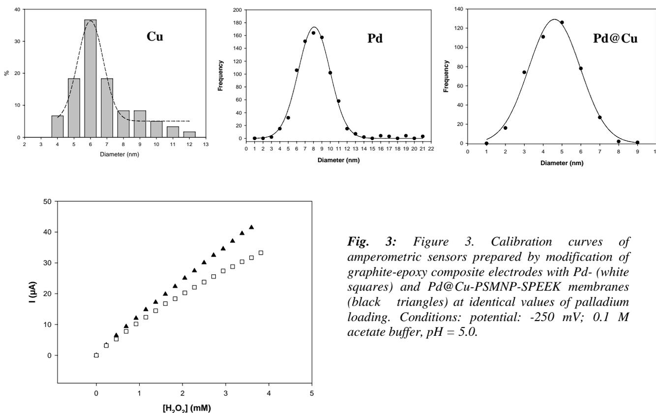
*Fig. 3: Figure 3. Calibration curves of amperometric sensors prepared by modification of graphite-epoxy composite electrodes with Pd- (white squares) and Pd@Cu-PSMNP-SPEEK membranes (black triangles) at identical values of palladium loading. Conditions: potential: -250 mV; 0.1 M acetate buffer, pH = 5.0.*
