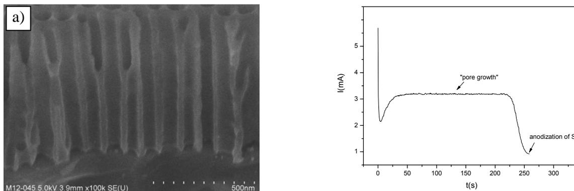
Fig.2: Realization of opened bottom pores on top of a *n*-poly-Si layer by highly controlled anodization. a) SEM image of the alumina membranes with open pores on *n*-poly-Si layer; b) current characteristics during anodic oxidation.
