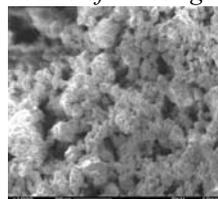
Fig.4 SEM microstructure of PT sol-gel powder (C sample)
