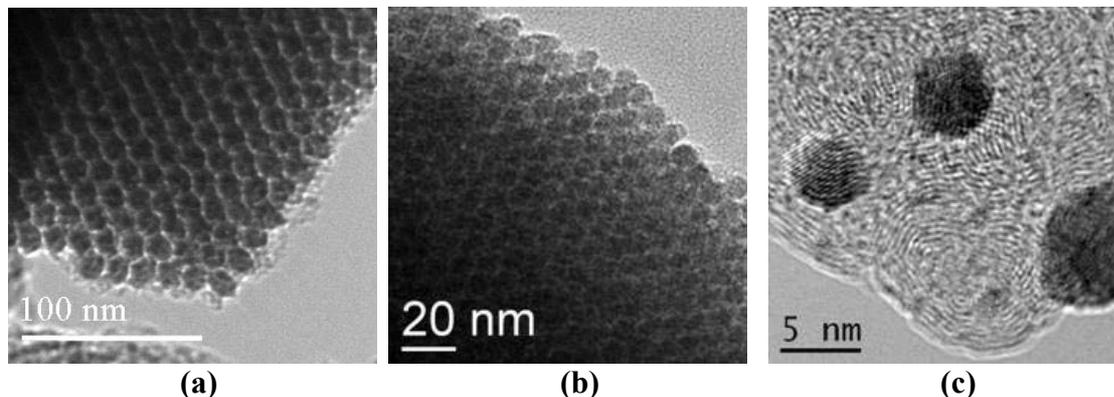
Fig. 1. TEM micrographs: (a) CMK-3 carbon, (b) CMK-3 carbon treated with  $\text{HNO}_3$  (from ref. 1 and ref. 2, respectively), and (c) PtRu supported nanoparticles.
