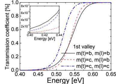
**Fig. 12:** Transmission coefficients as a function of energy at  $V_G=0.15 \text{ V}$  and  $V_D=0.05 \text{ V}$  in the 6 nm gate length, 1.3 nm thick body DG MOSFET. The inset shows the detailed onset of the transmission.
