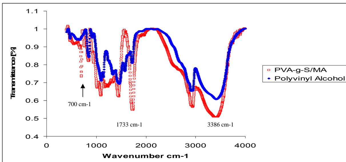
Figure 1. FT-IR spectroscopy of copolymer of styrene - maleic anhydride which is grafted on polyvinyl alcohol (PVA-g-S/MA) & pure polyvinyl alcohol (PVA).
