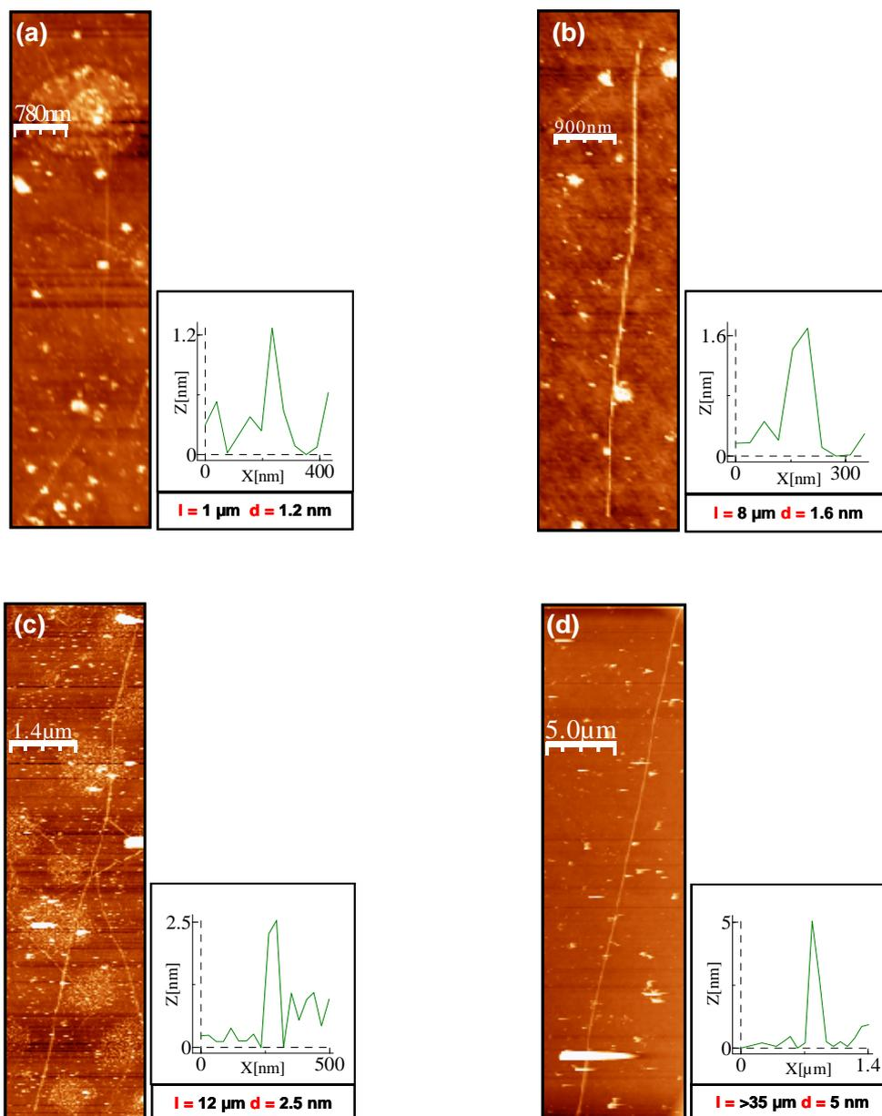
**Figure 1** AFM topography images of SWNT growth by CVD on silicon substrates:
