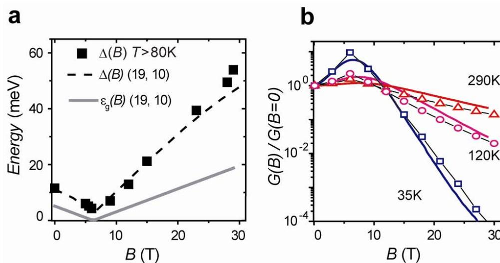
**Figure 3.** (a) Transport activation energies  $\Delta(B)$  determined from the conductance Arrhenius plots (sample 1) and  $\Delta(B)$  calculated for the (19,10) CNT. Gray line shows calculated  $\epsilon_g(B)$  dependence. (b) Solid lines show simulation results for the (19,10) CNT. (b) Normalized off-state magnetoconductance of sample 1 compared to simulations for the (19,10) CNT.
