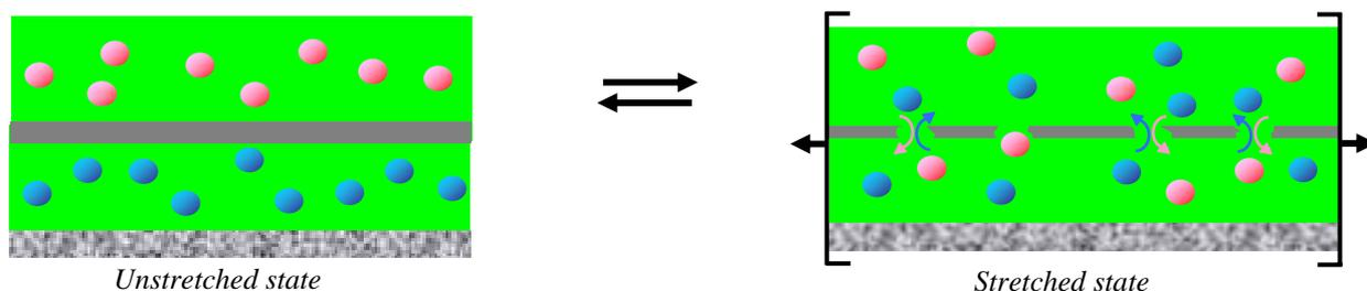
*Schematic representation of a multicompartiment film before and during the stretching state. The gray line corresponds to the barrier that allows diffusion of molecules from one compartment to the other when the stretching is applied and nanopores are formed.*
