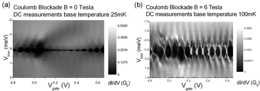
FIG. 3: (a) Differential conductance at zero magnetic field with superconducting electrodes. (b) Differential conductance for the same gate voltage region as in (a) but with a magnetic field of  $B = 6\text{T}$  in order to drive the electrodes into the normal state.
