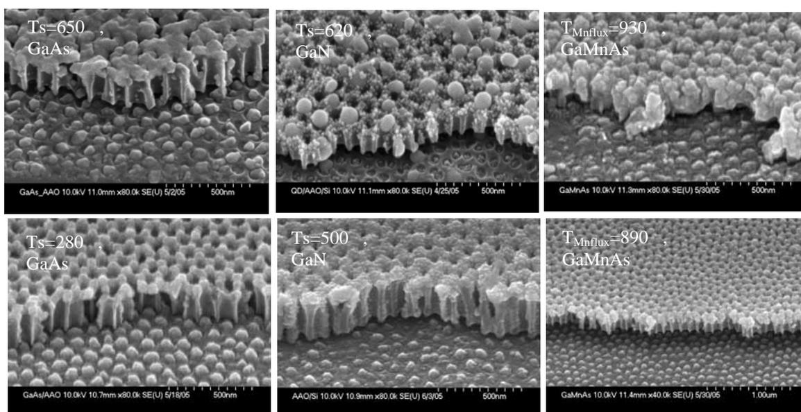
Fig. 2 SEM images of nanodot arrays of GaAs(left), b)GaN(center), and GaMnAs(right) with AAO templates.
