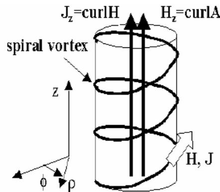
Fig. 2. Model of a magnetic vortex in generally accepted geometrical representation shown in cylindrical coordinate system  $(r, j, z)$
