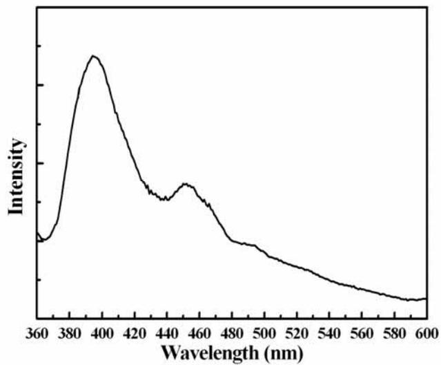
Fig. 2. PL spectra of ZnO nanowires synthesized in ITO glass substrate.
