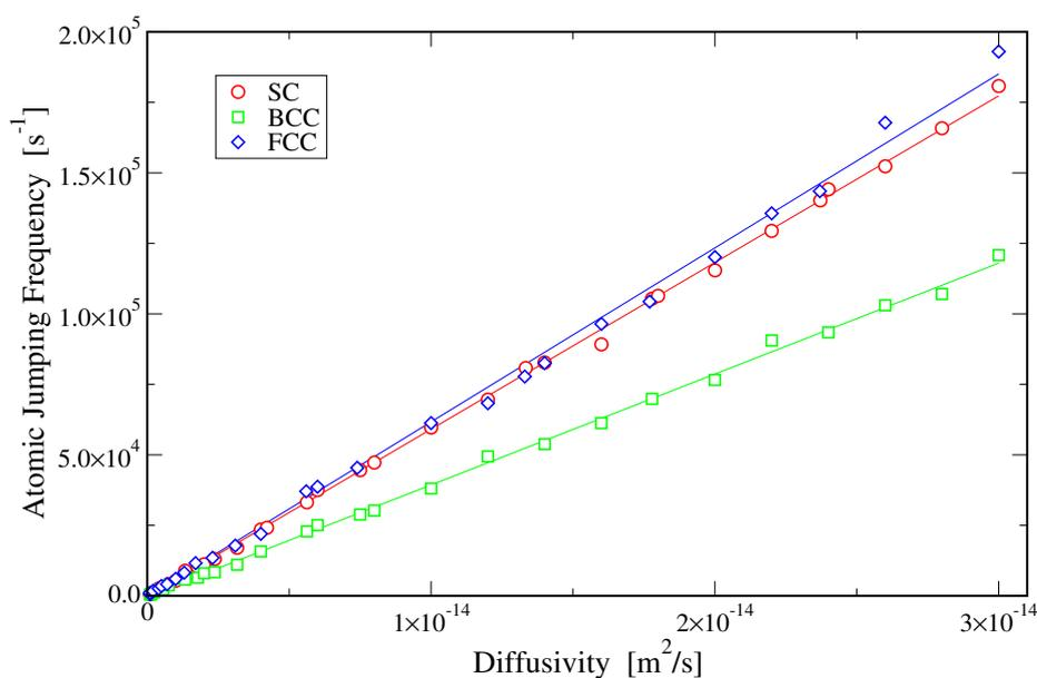
**Figure 1:** Atomic jumping frequencies needed to simulate different diffusivities for SC, BCC and FCC lattices, for a cell size of 1 nm.
