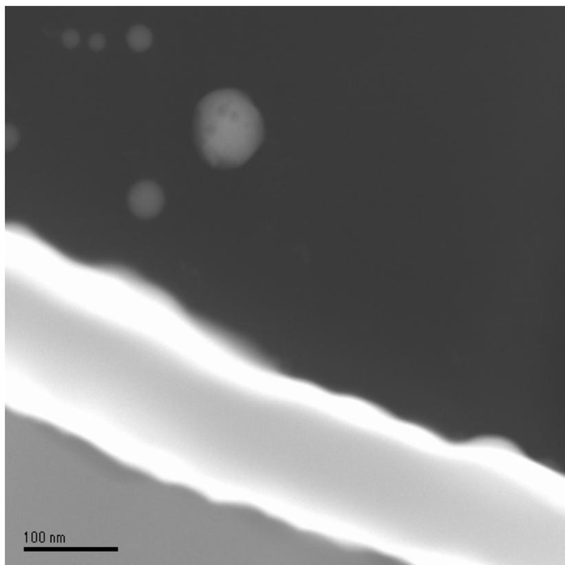
**Figure 1** A TEM image of a single  $\sim 62$  nm wide  $\text{Sm}_2\text{Fe}_{17-x}\text{Ta}_x\text{N}_{3-\sigma}$  nanodroplet on a Si substrate sputtered with Ta. Four 15 nm nano-crystal islands were grown on the top of the Ta substrate surrounded by the amorphous material.
