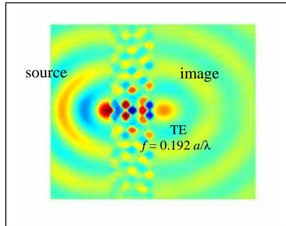
Fig.2 Snapshot of the (TE)  $H_z$
