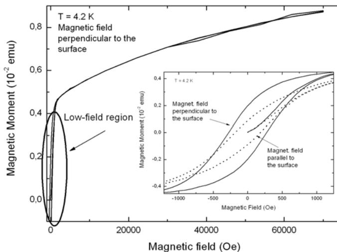
Magnetization curves of a Ni-filled sample exhibiting a non-saturating magnetic behavior at high magnetic fields far above the saturation magnetization of Ni (0.62 T). In the inset the hysteresis loops for easy axis and hard axis magnetization at low magnetic fields are shown.
