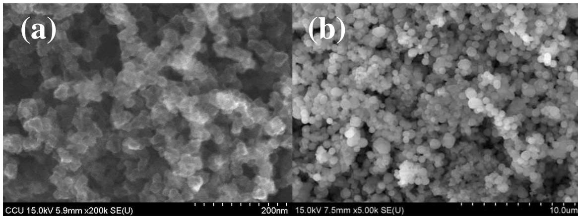
Figure1. SEM of as-synthesized (a) carbon nanocapsules and (b) SiO<sub>2</sub> spheres
