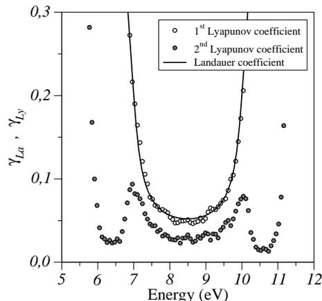
FIG. 1:  $2/3$  of Landauer exponent  $\gamma_{La}$  (solid line) and the largest Lyapunov exponent  $\gamma_{Ly}$  (white circles), as a function of energy, for  $t_{\perp} = 0.5$  eV and  $t_{\parallel} = 1.0$  eV. The second, smaller Lyapunov exponent (grey circles) is also shown.
