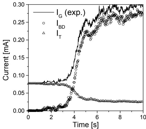
Fig. 3. Progressive breakdown current during a constant voltage stress at -3.75 V.
