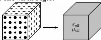
Fig. 1 A composite construct with two sets of dielectric spheres. If the wavelength is much larger than the radii of the spheres and the distance between them.
