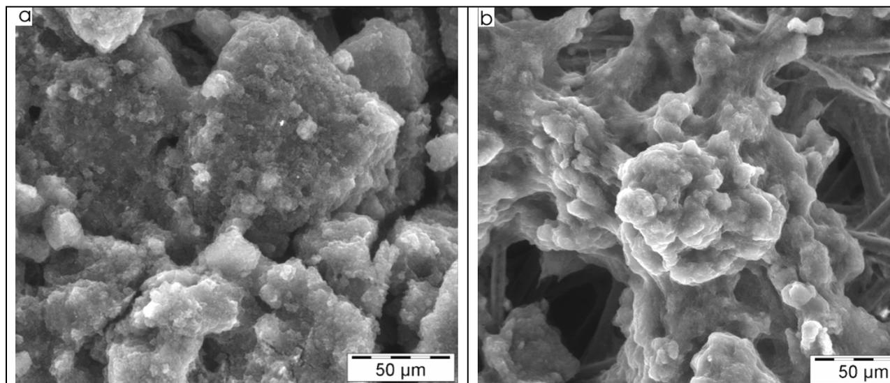
**Figure1.** Scanning electron microscopy images of biofilm growth on: a) carbon aerogel and b) MWNT
