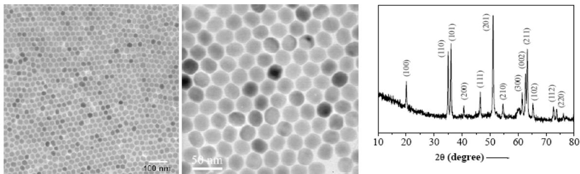
Figure 1 TEM images and XRD pattern of hexagonal-phase  $\text{NaYF}_4$ : Yb, Er/Tm nanocrystals
