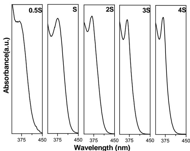
**Figure 1.** Absorption spectra of CdS NCs prepared at different degree of supersaturation
