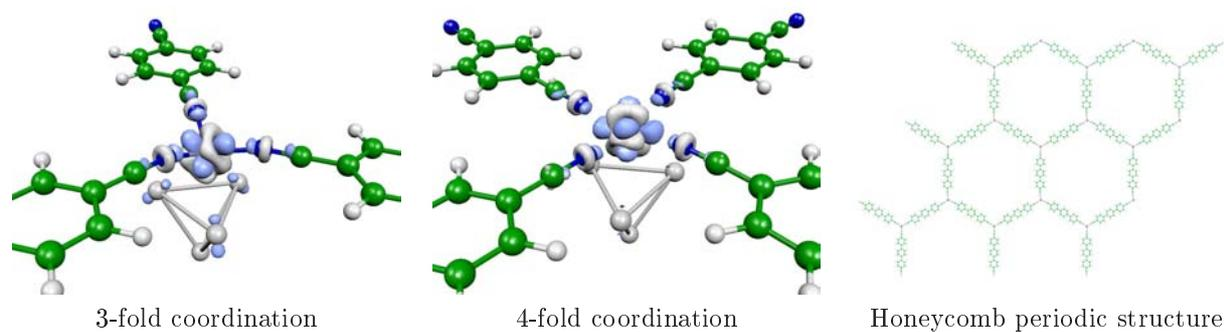
Figure 2: Induced charge density plots around the cobalt atom for 3-fold and 4-fold coordination. The corresponding honeycomb lattice for the 3-fold coordination is also shown.
