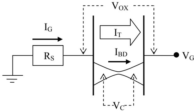
Fig. 1. Equivalent circuit model for the broken down MOS capacitor. The hourglass-like structure represents the breakdown path.
