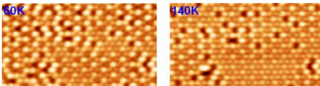
**Figure 1:** STM images of the same region ( $22 \times 12 \text{ nm}^2$ ) extracted from a movie showing the immobility of defects in the 60K-140K interval of temperatures. Tunneling parameters for both images:  $V_s = -1.5 \text{ V}$ ;  $I = 0.1 \text{ nA}$ .
