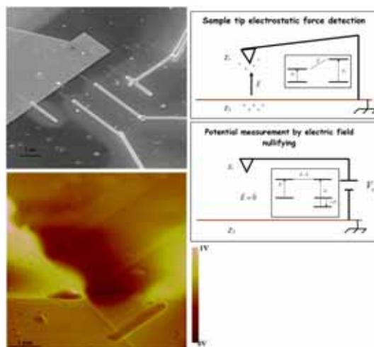
**Figure 1** Top : SEM image of a MWCNT contacted by ion beam induced platinum deposition. Two separated groups of halos can be identified. The inset shows the principle of KFM imaging. Bottom: Kelvin force Microscopy image of the biased MWCNT (here through the outer electrodes), showing surface potential distribution along the nanotubes. Each group of halos is seen to be equipotential.
