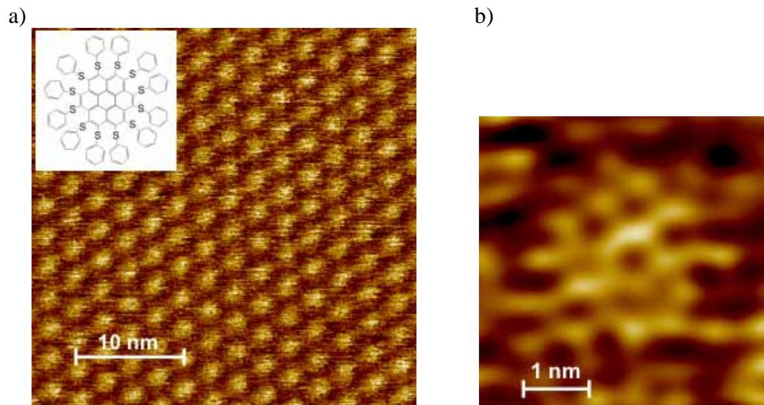
**Fig. 1** STM images showing a) the hexagonal structure of a self-assembled layer of dodecakis(phenylthio)coronene (inset: chemical structure of the molecule) and b) the molecule in submolecular resolution.
