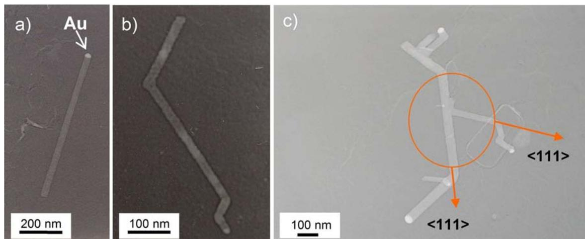
**Figure 2:** a) Monocrystalline silicium nanowire observed with TEM.
