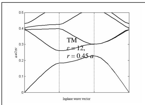
Fig.3 Band structure, TM
