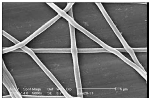
Fig.3. SEM micrograph of 10wt% PANi (25Kvs)
