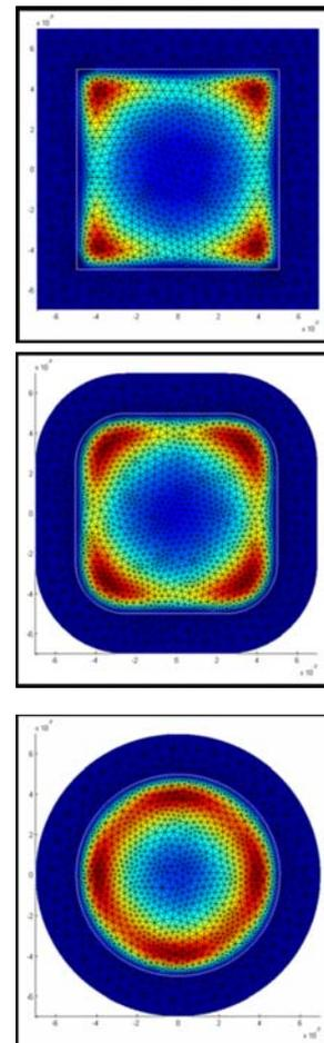
**Figure 4.-** Electron density in silicon QWIs with variable cross-section, from square to circular.
