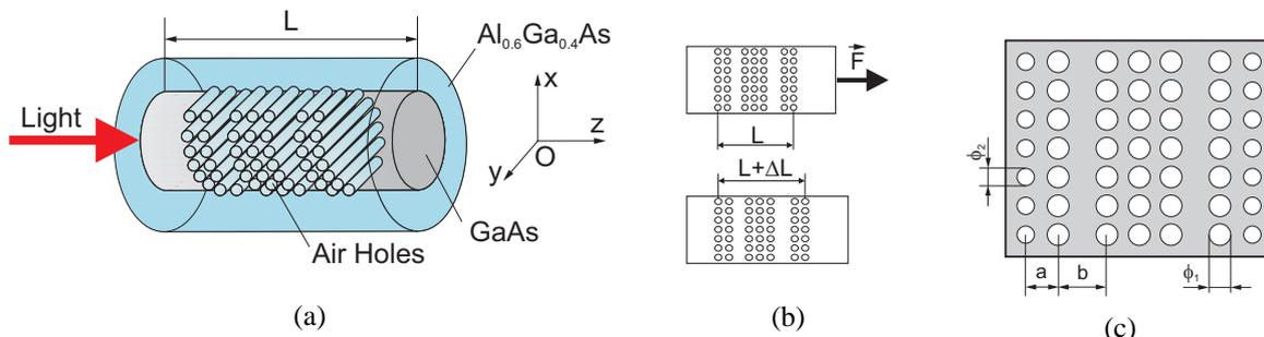
Fig. 1. (a) Schematic view of the PC sensor embedded in a FO; (b) Deformation of the sensor of length  $L$ , under a loading force  $F$ ; and (c) A section through the PC (air holes) showing the elementary geometrical dimensions  $a$ ,  $b$ ,  $\phi_1$ ,  $\phi_2$ .
