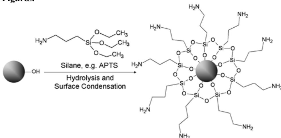
**Figure 1:** Silanisation of silica-magnetite nanoparticles.
