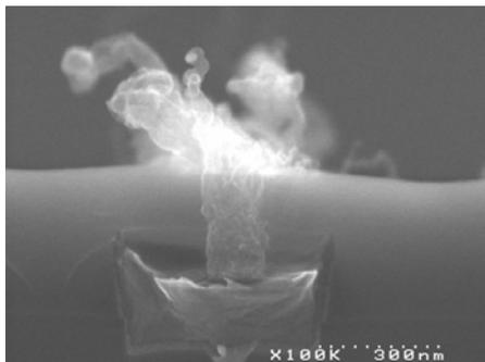
Fig.c: SEM cross section of a 140nm wide via on a copper line. Surrounding dielectric is silicon dioxide. Nanotube density is  $5.10^{10}$  CNT/cm<sup>2</sup> per via.
