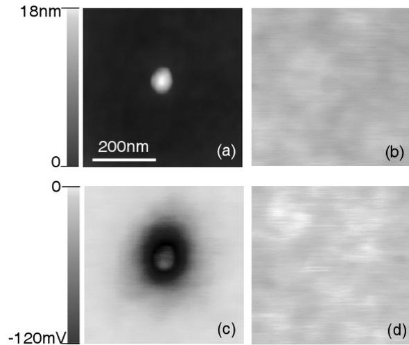
**Fig.2** Topographic image (a) and corresponding surface potential images of an isolated Si dot with a Ge core measured by AFM/Kelvin probe mode before (b) and after electron injection (c) at -3V, and after electron emission at +1V from the charged Si dot in the tapping mode (d).
