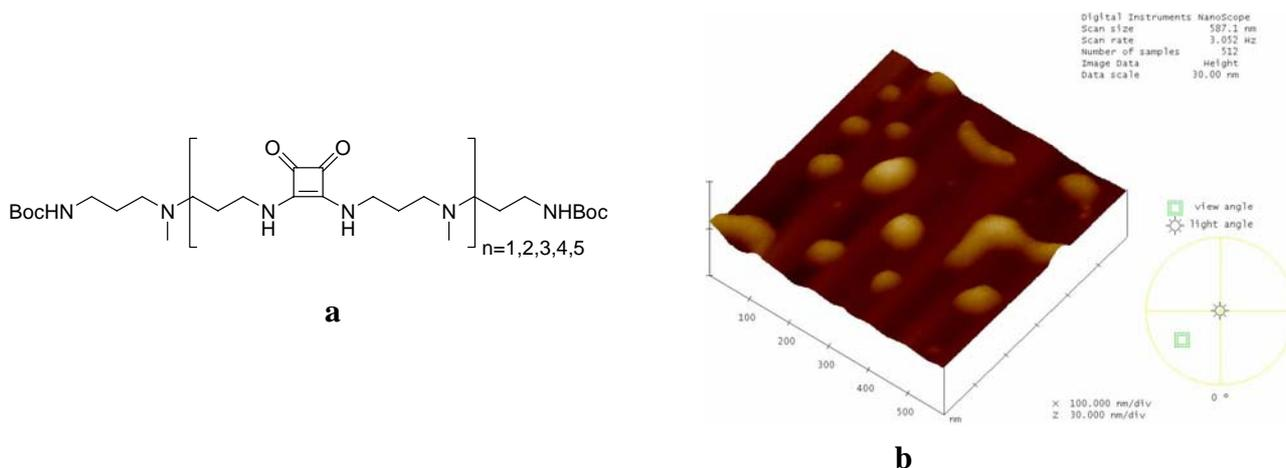
**Figure 1. a) general structure of oligosquaramides. b) AFM image of globular nanostructures of oligosquaramide n=5**
