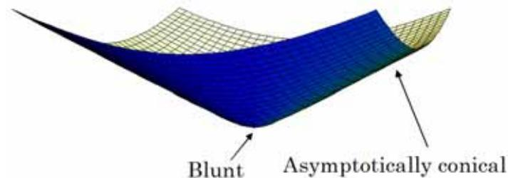
Figure 1. A real tip looks like a cone at large scales, but like a sphere at small scales.
