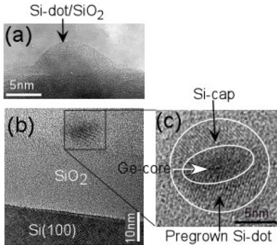
**Fig.1** Cross-sectional HR-TEM images of hemispherical Si dot pregrown on SiO<sub>2</sub> (a) and Si dots with Ge core (b) accompanied with a magnified image of an isolated dot (c).
