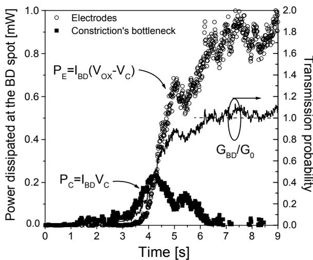
Fig. 5. Power dissipated at the PBD spot as a function of time.
