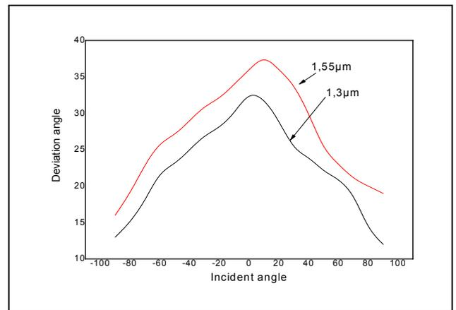
Fig. 3 Angular dispersion angles for various incident angles for TE and TM polarisation
