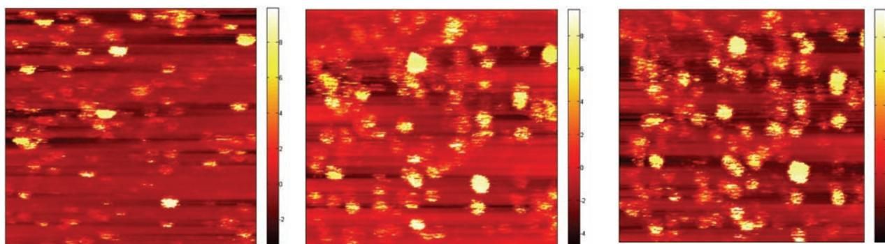
Figure 3. Consecutive current maps at 5V on the same area of a high-*k* sample. The measurements were performed in vacuum. The same experiments can not be reproduced in air without loss of tip conductivity.
