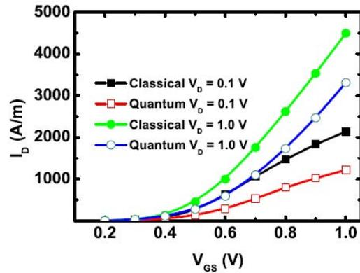
**Figure 3.-**  $I_D$ - $V_{GS}$  curves comparison calculated for  $V_{DS}=0.1V$  and  $1V$  when classical and quantum description are used.
