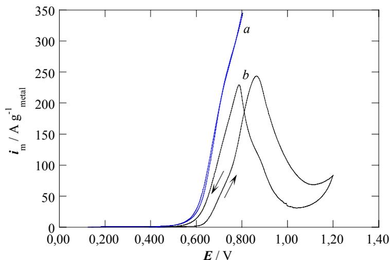
Fig. 2. Cyclic voltammograms of methanol oxidation on DMFC anodes catalyzed by: (a) PtRu/CMK3-Nc0.5 and (b) Pt/CMK3-Nd0.5, in 2.0 M  $\text{CH}_3\text{OH}$  + 0.50 M  $\text{H}_2\text{SO}_4$ .  $T = 60^\circ\text{C}$ .  $v_b = 20 \text{ mV s}^{-1}$ .
