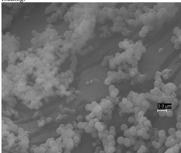
Fig. 2. Scanning electron microscopy image of PS-VBC-DVB with nanoparticles loaded at 1% by mass to the amount of monomer.
