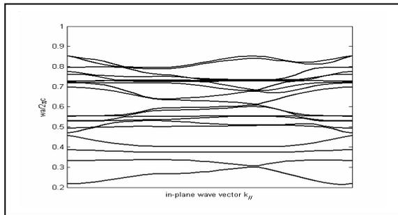
Figure 1. Band structure of the PC with 4 Si/SiO<sub>2</sub>
