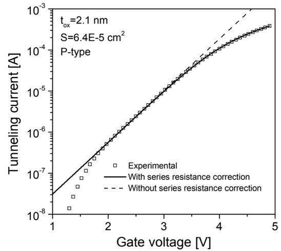
Fig. 2. Tunneling current through the fresh device.
