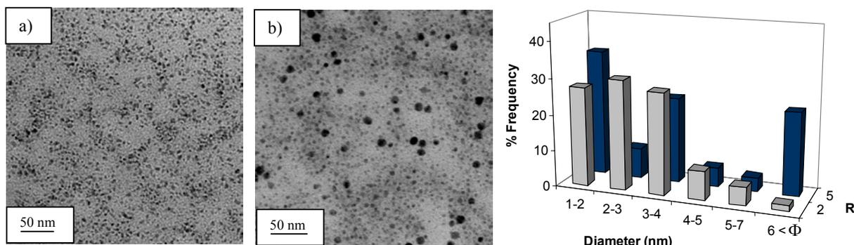
**Figure 3.** TEM photographs and the corresponding particle size distribution histograms obtained when mixing a stoichiometric amount of  $\text{CuCl}_2$ -containing microemulsions  $\{[\text{CuCl}_2] = 3.0 \text{ mM}, [\text{AOT}] = 200 \text{ mM}, (a) R = 2.0; (b) R = 5.0\}$  with  $\text{NaOH}$  for 3 h at 300 rpm.
