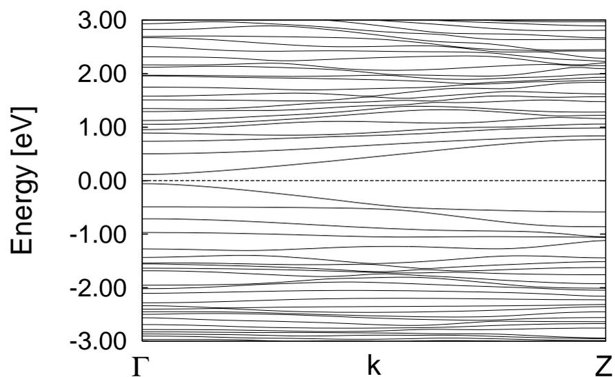
FIG. 3: Band structure of a (10,0) CBNNT showing the existence of a gap, which is reduced in numerical value with respect to its pristine CNT analogue.
