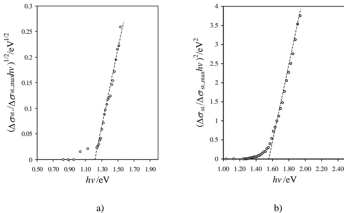
Fig. 1. Determination of the indirect (a) and direct (b) band gap energies for a nanocrystalline tin(II) selenide film sample on the basis of its photoconductivity spectrum using the parabolic approximation for the dispersion relation.
