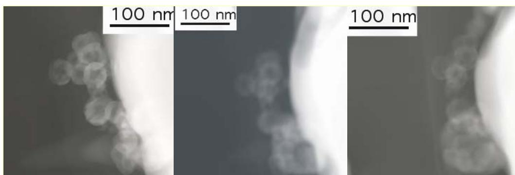
**Figure 2.** TEM image of clusters of  $\text{Sm}_2\text{Fe}_{17-x}\text{Ta}_x\text{N}_{3-\sigma}$  nanodroplets on a Si substrate coated with Ta.
