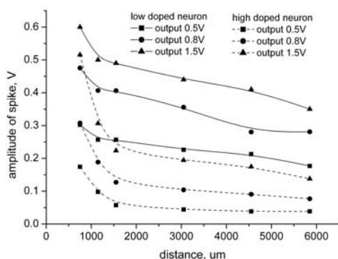
Fig.2. The attenuation of spike amplitude with wire distance dependent on output voltage. Diffusion lengths are 2 and 4 mm for low and high doped neurons respectively.
