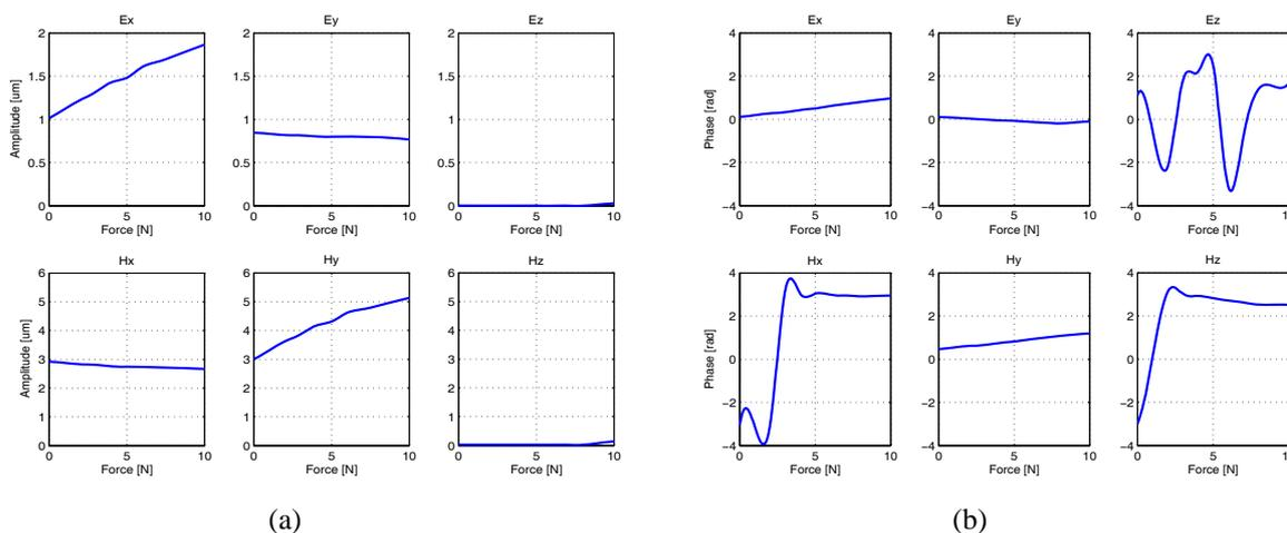
Fig. 2. (a) Amplitude ( $\vec{E}$  and  $\vec{H}$ ) versus elongating (loading) force  $F$ ; (b) Phase ( $\vec{E}$  and  $\vec{H}$ ) versus elongating (loading) force  $F$ .
