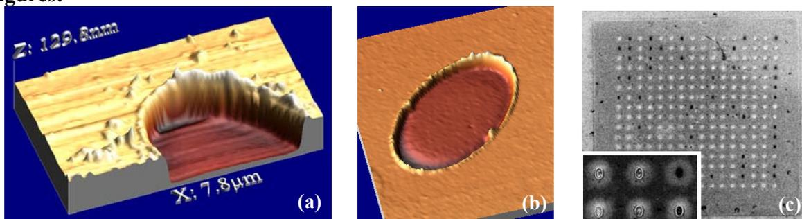
Fig. 1: (a) and (b) Atomic force microscopy images of an empty elliptical antidot and a filled one respectively both patterned on  $\text{Co}_x\text{Si}_{1-x}$  thin film. (c) SEM image of a square array of elliptical fill antidots. The inset shows that more than the 80 % of the antidots are filled.
