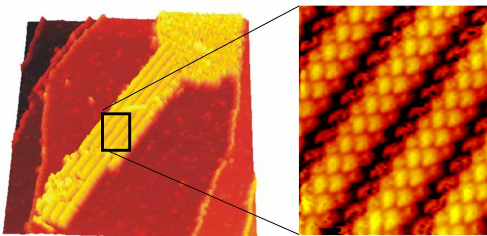
**Figure 2.**  $98.4 \times 98.4 \text{ nm}^2$  STM image of long tubes coexisting with disorder after depositing ZnTMP on Cu(100) and a zoom-in showing the spiral shape of the tubes
