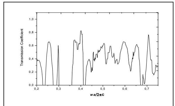
Figure 4 Transmission of the PC with 8 pair Si/SiO<sub>2</sub>
