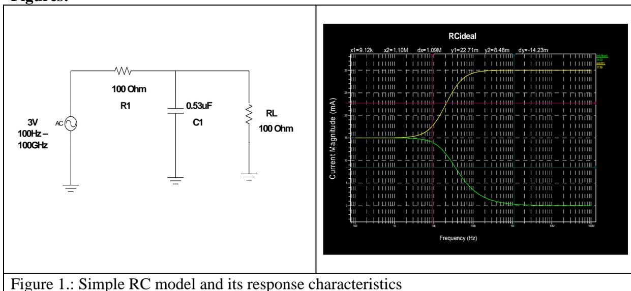
Figure 1.: Simple RC model and its response characteristics
