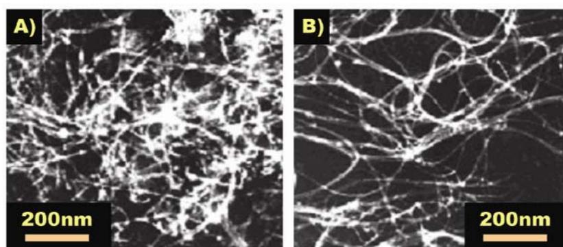
**FIGURE 2.** The SEM images of CNTs A) before B) after purification stage
