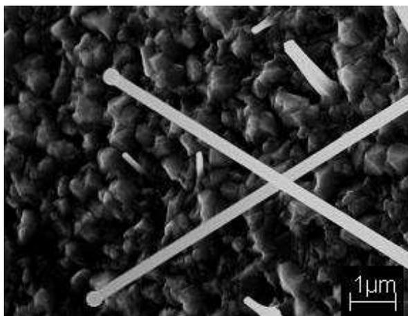
**Fig. (2).** SEM image of self-catalyzed GaAs grown on cleaved edge of Si (100). NWs have Ga droplet at the top demonstrating self-catalyzed growth and nanorods are also present with no droplet at the top.
