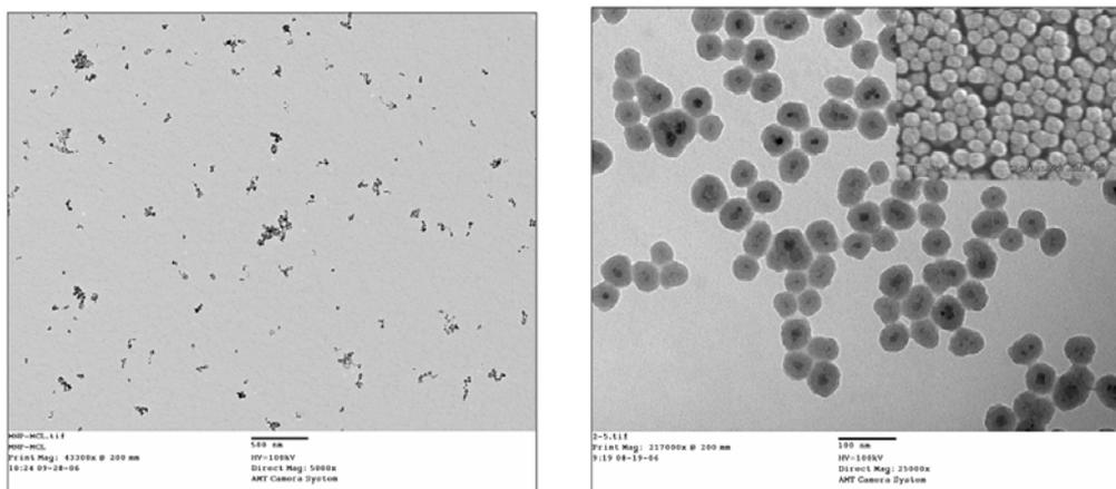
Figure 1. TEM images of synthesized cobalt ferrite nanoparticles (left) and silica coated nanoparticles (right)
