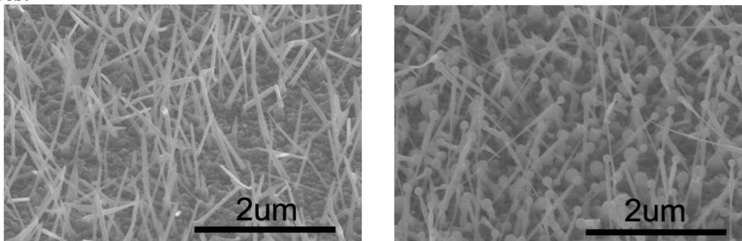
Figure 1. SEM images of ITO nanowires grown (a) with oxygen and (b) without oxygen.
