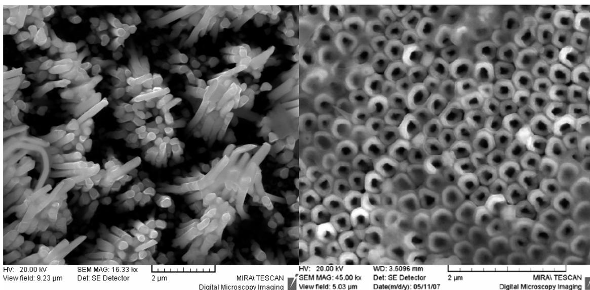
**Fig.2:** Nanowires**Fig. 3:** Nanotubes
