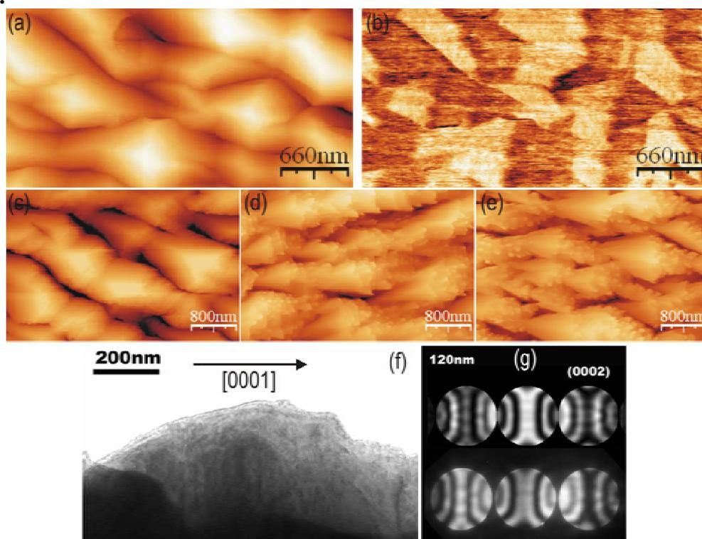
**Fig 1:** (a) SFM topography and (b) KPM images of a ZnO thin film sample grown along the  $[11\bar{2}0]$  direction. Topography images of the same sample etched (c) 30s in a 0.01M, (d) 5s in a 0.1M and (e) 10s in a 0.1M HCl solution. (f) TEM image of an etched pyramid and (g) CBED patterns (simulated and experimental) establishing the absolute polarity of the pyramid.
