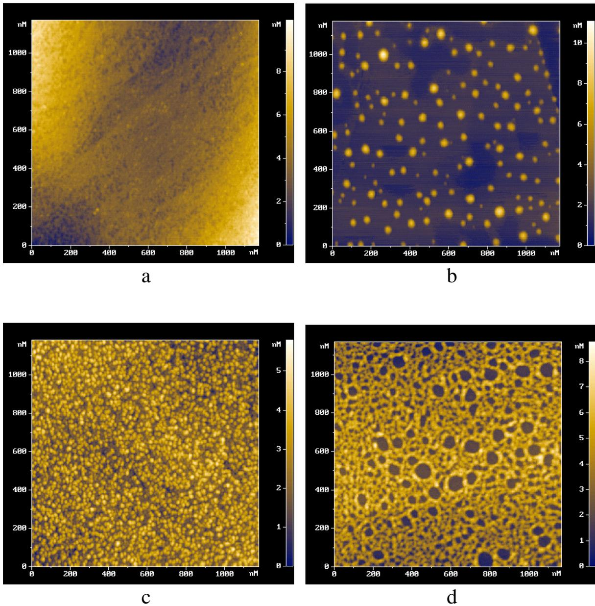
SFM images of nanofilms: a) PPh on HOPG surface; b) poly((dimethyldiallylammonium) chloride) (PDDA) on HOPG surface; c) antibodies on PPh film (HOPG); d) antibodies on PDDA film (HOPG).
