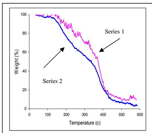
Figure 2. STA experiments of nanocomposite (series 1). & PVA-g-S/MA (series 2).
