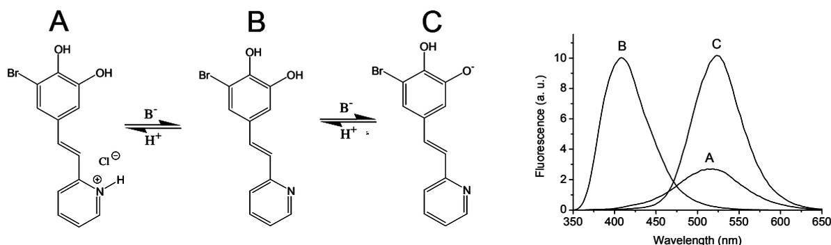
Figure 1. Catechol-based switch, (left) states of the molecule, (right) fluorescent spectra.
