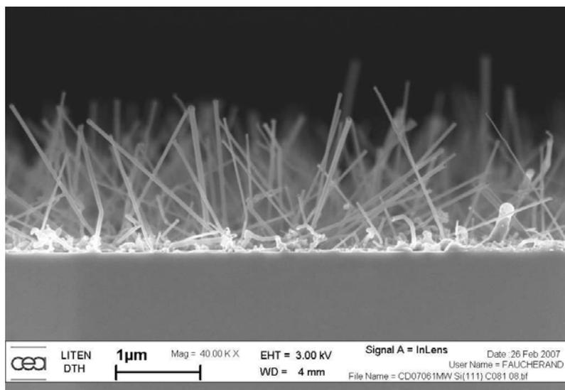
**Figure 1: Silicium nanowires (diameter ~50nm) from gold colloids.**
