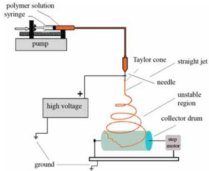
Figure 1. Schematic of electrospinning set up for producing nanofiber.
