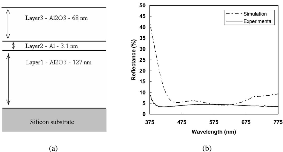
**Figure 1.** (a) Schematic showing an Al<sub>2</sub>O<sub>3</sub>-Al-Al<sub>2</sub>O<sub>3</sub> black mirror formed on silicon and (b) its simulated and experimentally obtained reflection characteristics.
