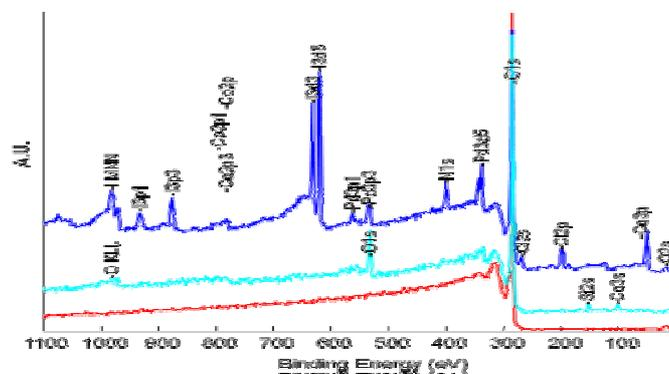
**Figure 3.** XPS spectrum of the surface of HOPG (red), the  $\text{CoPd}_2(\text{Me}_2\text{Ipz})_4\text{Cl}_4 \cdot 2\text{NH}_4$  before (blue), and after (clear blue) reduction process on HOPG.
