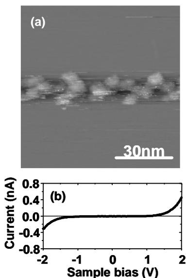
Fig. 1. (a) STM image of Co-BND deposited on HOPG. Observation conditions are:  $I_t = 0.15$  nA,  $V_{\text{sub}} = 1.7$  V. (b) I-V characteristic obtained from single Co-BND observed in Fig. 1(a).  $I_t = 0.15$  nA.
