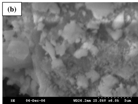
Figure 3. Scanning electron microscopy images of powder "S" (a) and "ZS" (b) thermal treated at 1000<sup>0</sup>C/2h
