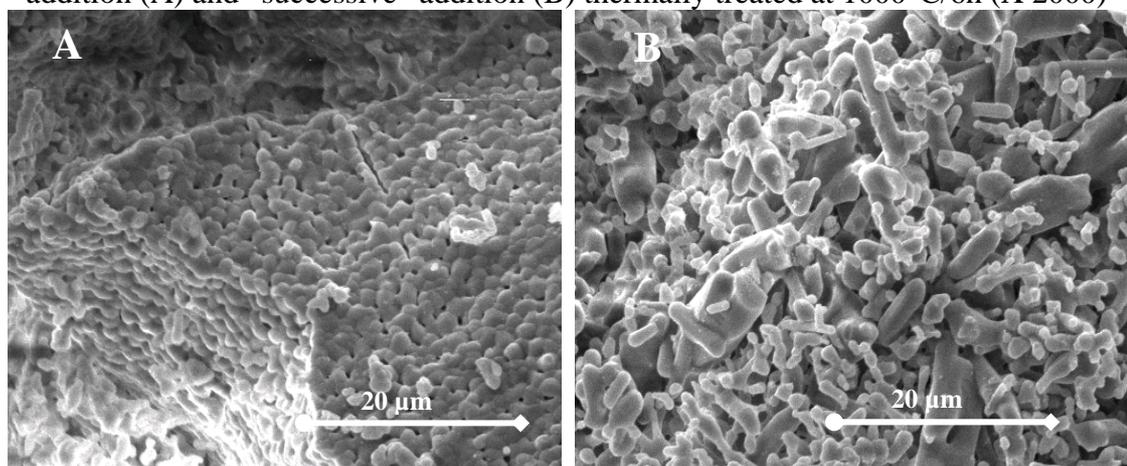
Figure 3: Scanning electron microscopy images of powder synthesized by “initial” addition (A) and “successive” addition (B) thermally treated at 1500°C/6h (X 2000)
