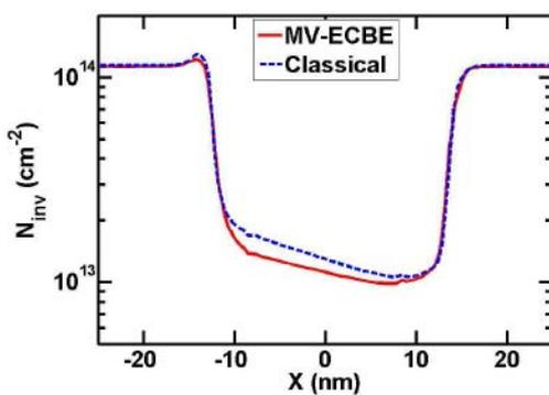
**Figure 2.-** Comparison of the inversion charge along the channel direction for classical (dashed) and MV-ECBE (solid) simulations. Quantum effects produce an increase in the threshold voltage
