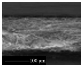
Figure 2. Scanning electron microscopy of cross sectional silk fibroin nanofiber mat.
