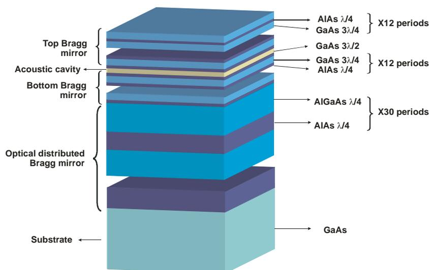
Figure 1: Scheme of the studied resonator for light and sound. The acoustic cavity acts as the spacer of the optical cavity.
