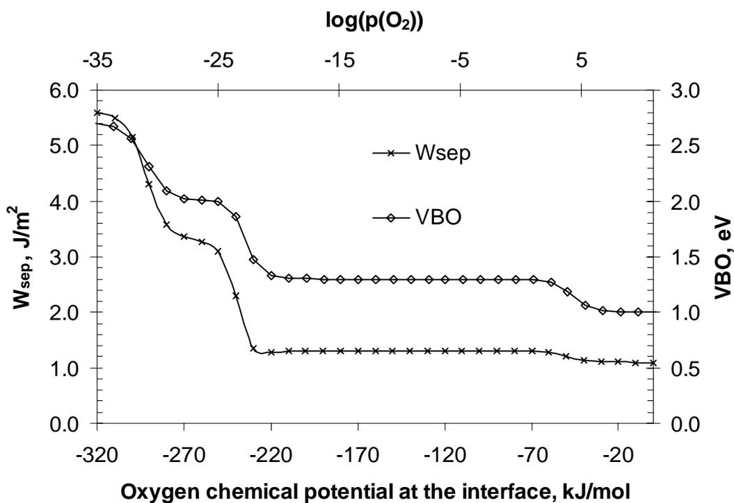
Fig. 2. Work of separation and valence band offset (VBO) for the Pt/HfO<sub>2</sub> interface as a function of the oxygen chemical potential at 500°C.
