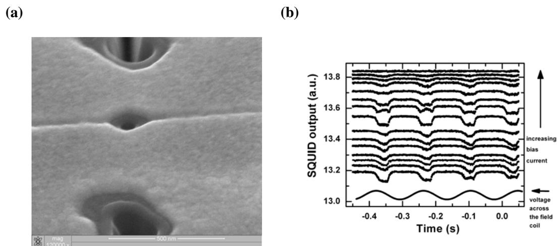
**Figure 1:** (a) Scanning electron micrograph of an Au-shunted Nb dc SQUID (scale bar: 500 nm) with an estimated loop diameter of about 50 nm. (b) Output of this device at different bias currents in response to an ac-modulated magnetic field applied perpendicular to the plane of the SQUID. The lowest trace is the ac modulation voltage, corresponding to a peak-to-peak field of 100  $\mu\text{T}$ .
