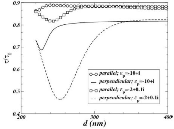
Fig. 2: lifetimes (normalized to its value in vacuum) for transition dipoles, parallel or perpendicular to a left-handed material slab with some absorption,  $\epsilon=-1+0.01i$  and  $\mu=-1+0.01i$ ; as a function of the distance between emitter and particle (placed on the other side of the slab). The remaining parameters are the same as in figure 1.
