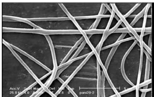
Fig.4. SEM micrograph of 20wt% PANi (25 Kvs)
