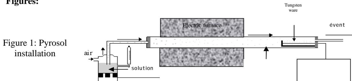
Figure 1: Pyrosol installation
