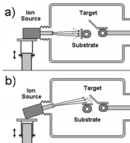
Fig.1. Schematic sketch of ion gun installation: a) substrate cleaning; b) ion beam sputter deposition.
