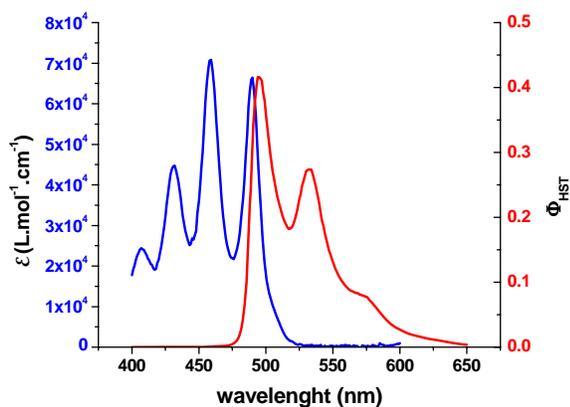
The extinction coefficient and normalized fluorescence spectrum versus wavelength of HST molecule dissolved in 98% dichlorobenzene.
