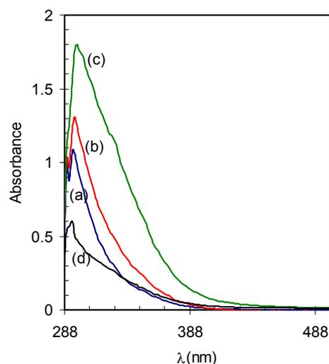
**Figure 2.** UV-absorption spectra of colloidal copper oxide nanoparticles obtained when mixing a stoichiometric amount of  $\text{CuCl}_2$ -containing microemulsions  $\{[\text{CuCl}_2] = 3.0 \text{ mM}, [\text{AOT}] = 200 \text{ mM}, (a) R = 2.0; (b) R = 3.0; (c) R = 5.0; (d) R = 8.0\}$  with  $\text{NaOH}$  for 3 h at 300 rpm.
