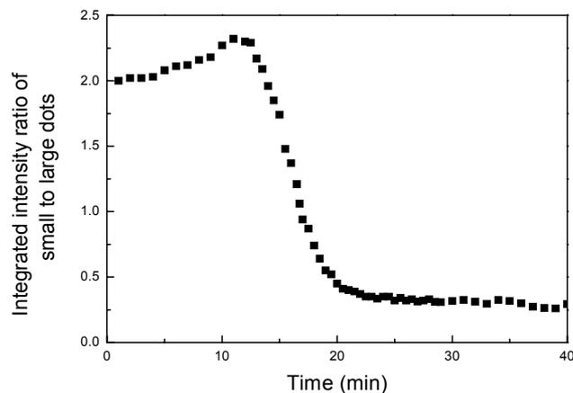
Fig.2: The variation of integrated intensity ratio of small to large dots with the increasing evaporation time.
