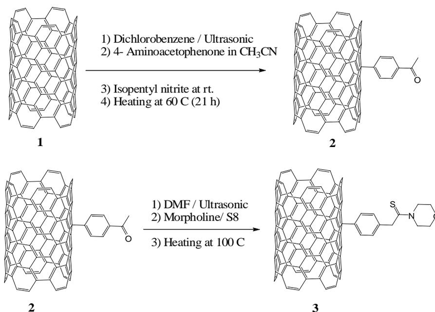
**Scheme 1.** Two steps reaction for the preparation of thioamide functionalized nanotube **3**.
