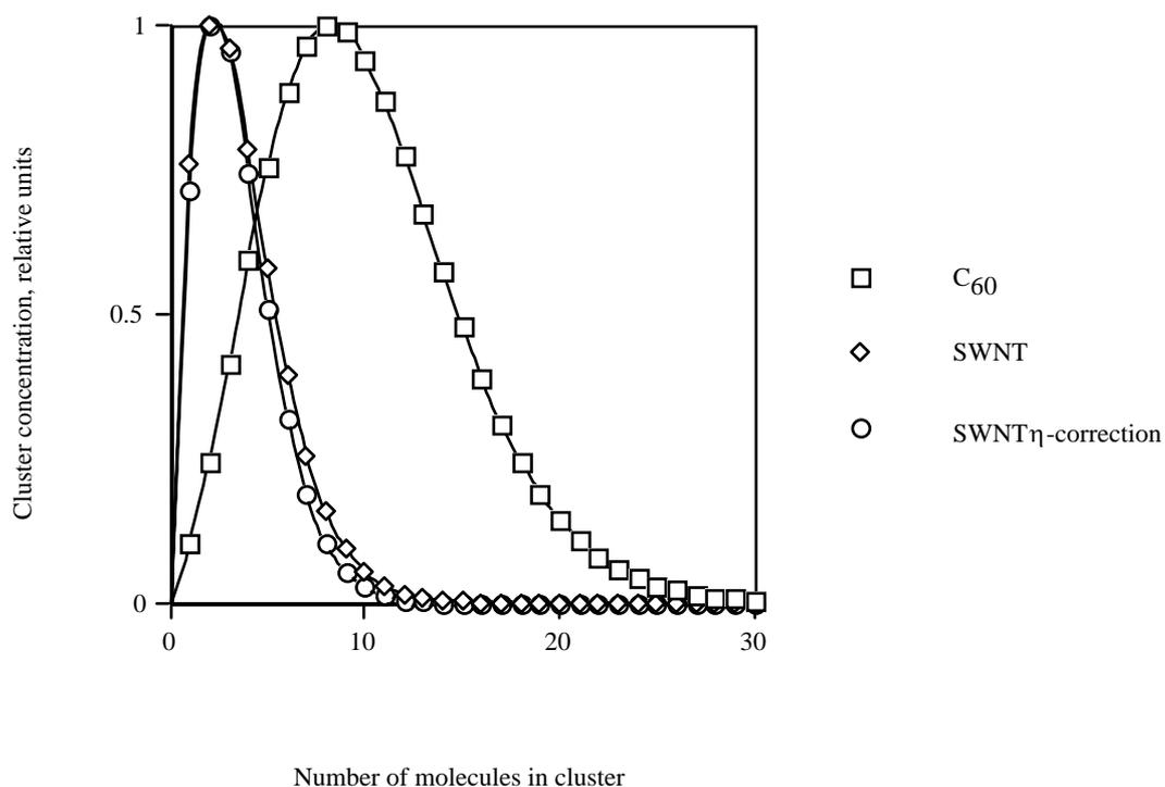
Fig. 2. Cluster distribution by size saturated in CS<sub>2</sub> at  $T = 298.15\text{K}$  of C<sub>60</sub> and SWNT.
