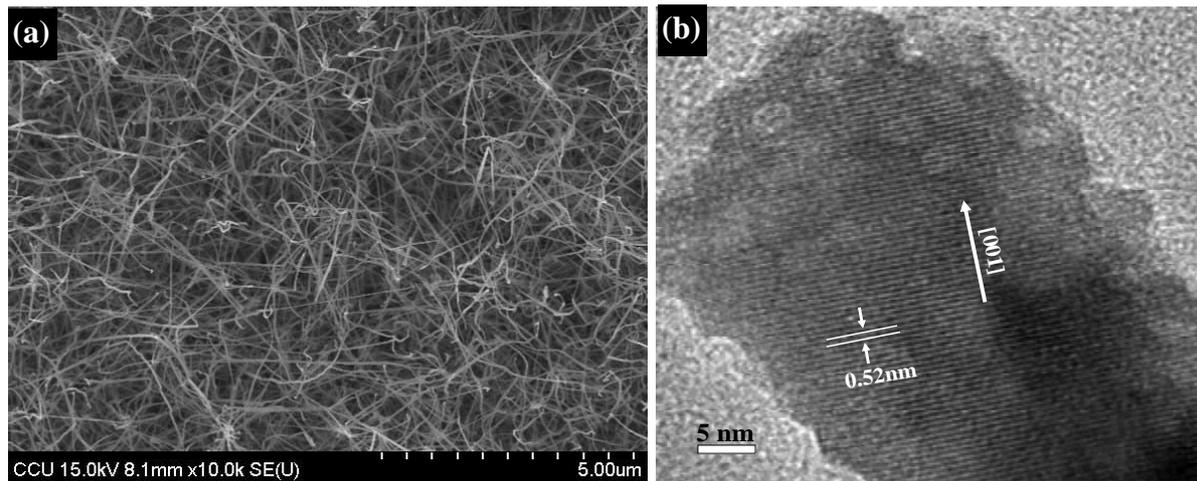
Fig. 1. (a) SEM and (b) HR-TEM image of ZnO nanowires.
