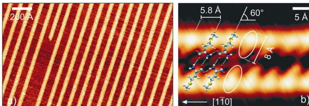
Figure 1 – STM images of the self-assembly of the *L*-methionine amino acid on Ag(111). (a) Regular and tunable 1D biomolecular nanogratings with a periodicity of  $94\text{Å}$  ( $I = 0.1\text{ nA}$ ,  $U = -500\text{ mV}$ ,  $\theta = 0.38\text{ ML}$ ). (b) Molecular resolution imaging shows molecular dimerization and commensurate growth along the closed-packed crystalline orientations ( $I = 0.9\text{ nA}$ ,  $U = -80\text{ mV}$ ).
