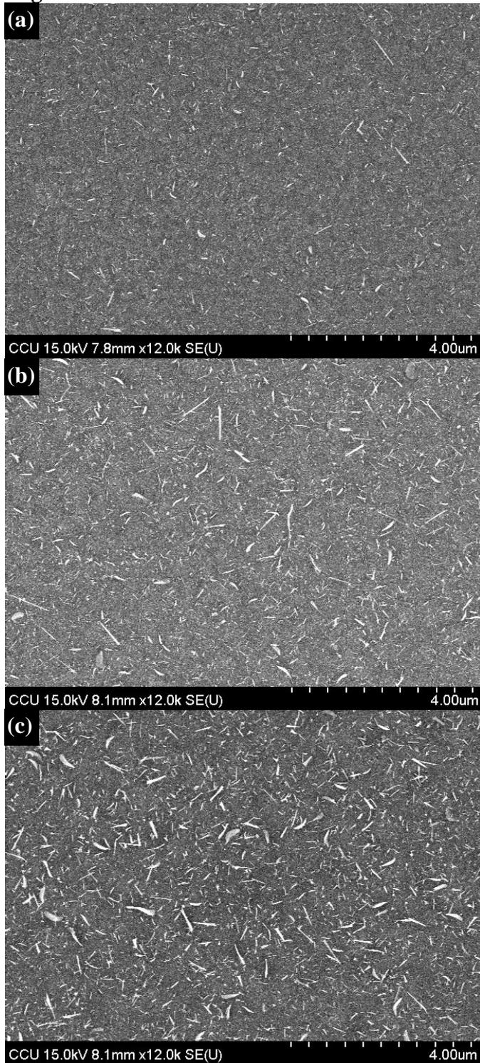
Fig. 1. FE-SEM of  $\alpha$ -Fe<sub>2</sub>O<sub>3</sub> nanowires growth on (a) 50nm, (b) 100nm and (c) 150nm of the iron films..
