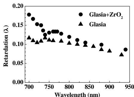
Fig. 2: Wavelength dependence of the retardation of the obtained wave plate made with ZrO<sub>2</sub>-dispersed Glasia® (circles) and Glasia® (triangles).
