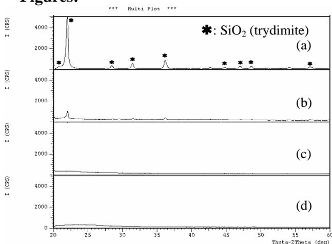
Figure 1. The spectrum of X-ray diffraction obtained on "S" powder, for various thermal treatments (a) 1200<sup>0</sup>C/2h; (b) 1100<sup>0</sup>C/2h; (c) 1000<sup>0</sup>C/2h; (d) as synthesized
