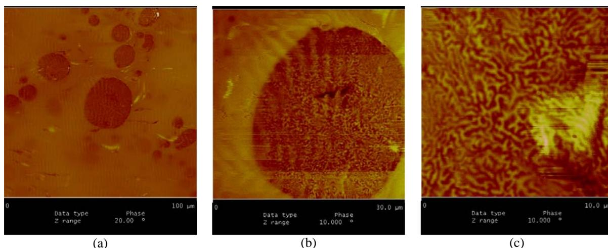
Figure 3.- MFM imaging of the as-received KUALMET powders at different magnifications (a) 100 x 100 μm (b) 30 x 30 μm (c) 10 x 10 μm.
