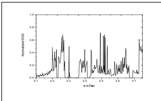
Figure 5 Density of state of the PC with 8 Si/SiO<sub>2</sub>
