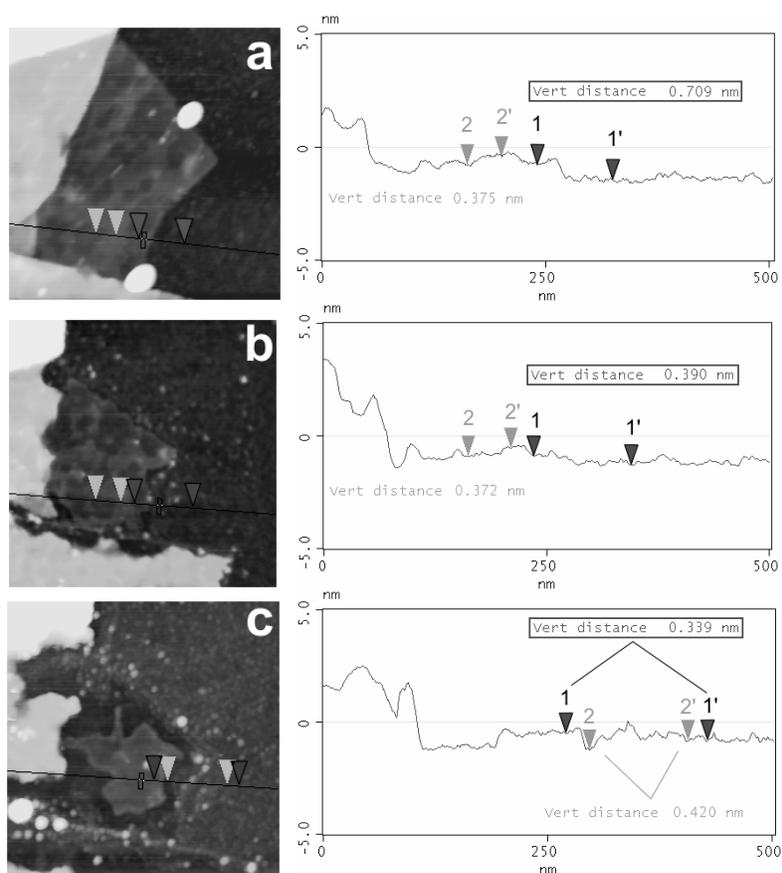
**Fig. 2.** AFM images of the same area of the few-layer graphite plate: (a) – after oxidation step I (450 °C for 10 minutes); (b) – after oxidation step II (550 °C for 10 minutes); (c) – after oxidation step III (550 °C for 20 minutes).
