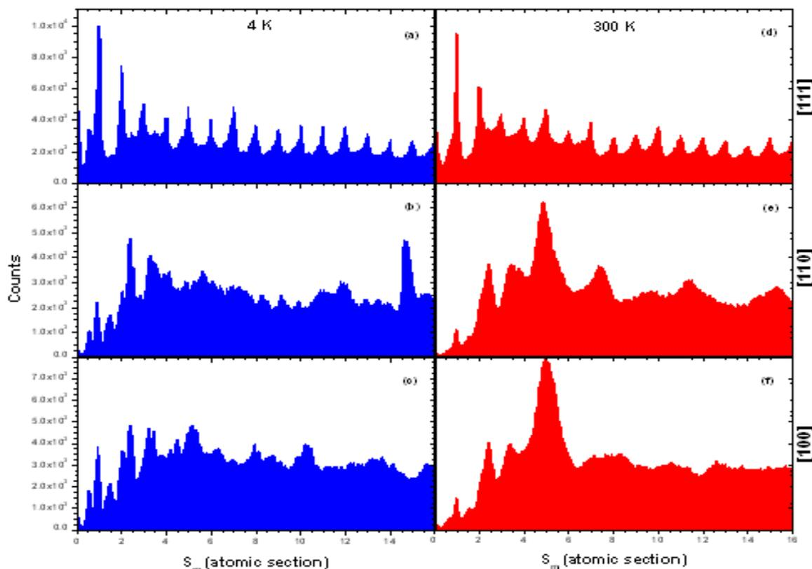
**Figure 1:** Minimum cross-section  $S_m$  histograms of Ni nanocontacts at  $T=4$  K (a,b,c) and 300K (d,e,f) evolving under stretching along the [111] (a,d), [110] (b,e), and [111] (c,f) orientations. Histograms have been built with 300 independent ruptures from the initial released parallelepiped of 390 (a,d), 420 (b,e) and 375 atoms (c,f).
