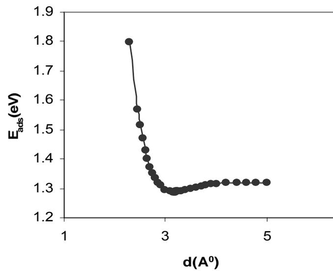
Figure 1: Typical adsorption energy (eV) as a function of tube molecule distance ( $\text{\AA}$ ) for  $\text{O}_2$  molecule on (5, 5) carbon nanotube.
