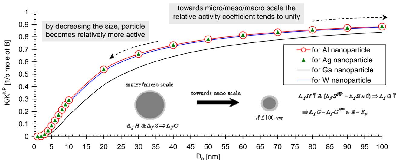
Fig. 2 Relative representations of size dependency effect on activity of Al, Ag, Ga and W nano-particles in a reactive medium.
