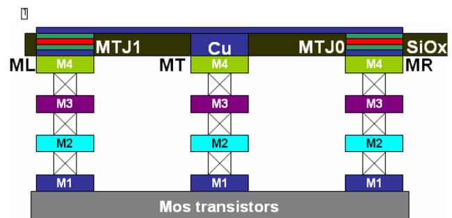
Fig.4 MTJ memory cells are implemented above the CMOS circuits
