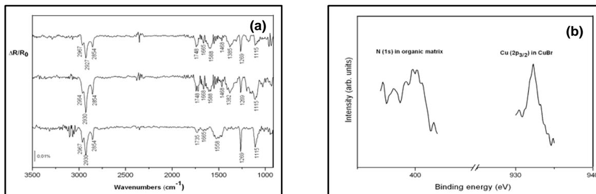
**Figure 2.** (a) PM-RAIR spectra after adsorption of  $[\text{CuBr}(\text{IN})]_n$  on gold from different adsorption methods. (b) XPS spectra after adsorption of  $[\text{CuBr}(\text{IN})]_n$  on gold surface.
