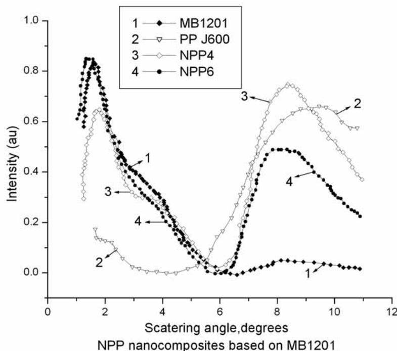
Fig.1 XRD pattern for NPP nanocomposites (1-10 degree)
