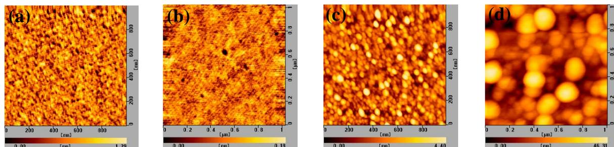
Fig. 2. AFM images of the surfaces of the co-deposited Fe-Sn catalyst (a) as deposited, (b) after annealing in air, (c) after heating to 700°C, and (d) after 1 s acetylene supply.
