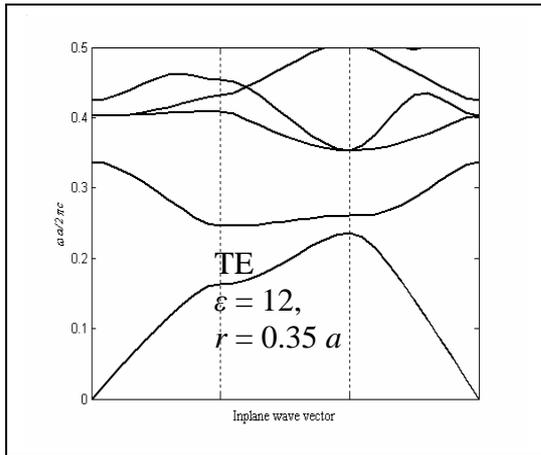
Fig.1 Band structure, TE
