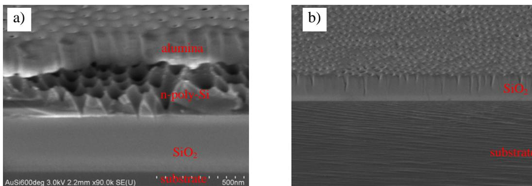
Fig.3: Porous alumina as etching mask for the *n*-poly-Si and  $\text{SiO}_2$  layers, SEM images. a) RIE etching at 30 W and 3 mTorr for 20 min; b) RIE etching at 50 W and 3 mTorr for 50 min followed by removal of the alumina membrane and *n*-poly-Si to show the transfer of the ordered structure (same sample as in a)).
