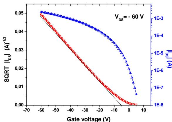
Transfer characteristics of a HST-OFET (deposition rate =  $0.2 \text{ A}^2/\text{s}$ , nominal thickness = 18 nm, W/L=18800/40  $\mu\text{m}/\mu\text{m}$ )
