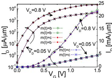
**Fig. 7:**  $I_D$ - $V_G$  characteristics for the 10 nm gate length DG MOSFET obtained from NEGF simulations. The impact of confined (c) masses in transversal  $[m(t)]$  and longitudinal  $[m(l)]$  transport directions is compared with that of bulk (b) masses.
