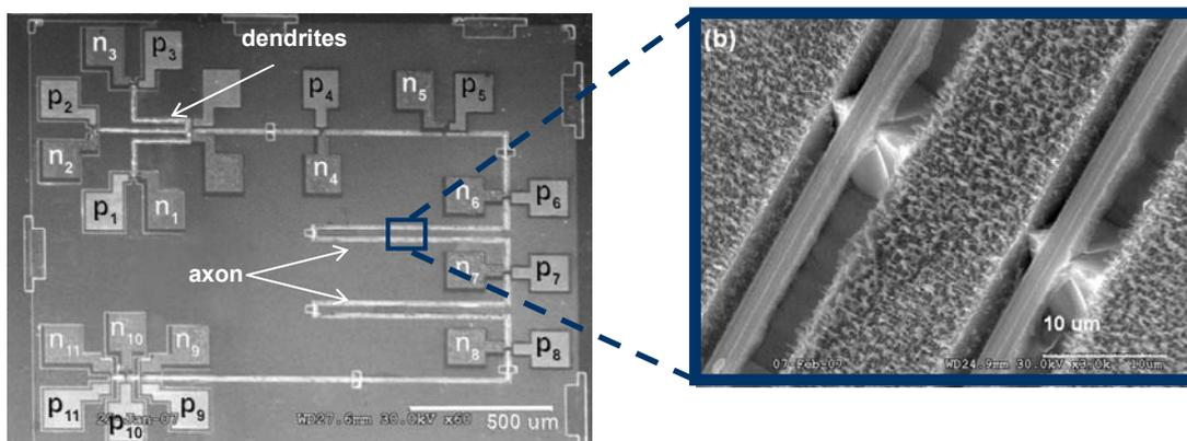
Fig.1. (a) – STM image of the GaAs-based neuron comprises of three dendrites, an axon and eleven pairs of Ohmic contacts ( $n_i, p_i$ ). (b) – The inset shows the fragment of the free-standing nanowire based on supporting bridges. The nanowire length is 6 mm, the width is 2  $\mu\text{m}$  and the thickness is 320 nm and 140 nm for low and high doped neurons respectively.
