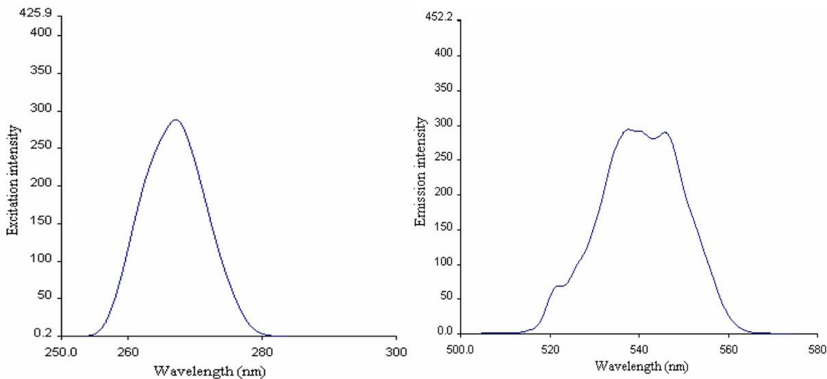
**Fig.2** Excitation and emission spectra of ZnS:Er
