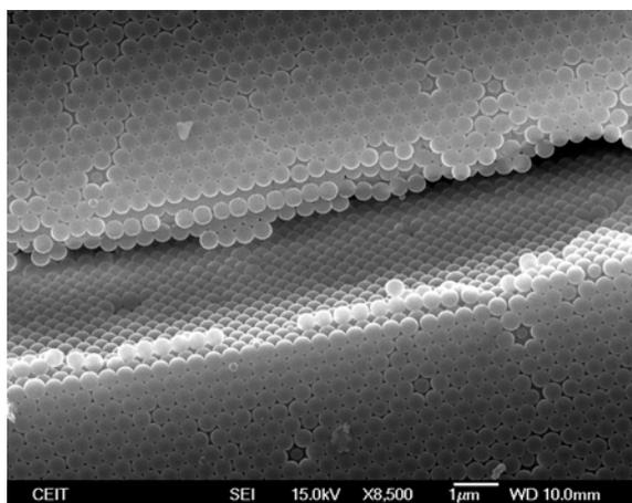
Figure 1. FEG-SEM micrograph of the insight of a crack in a 50 °C fabricated sample
