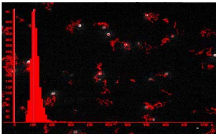
**Fig 1. A still from a video of 100nm polystyrene calibration particles showing *some* (for clarity) of the Brownian motion trajectories analysed and which is overlaid with the corresponding size plot.**
