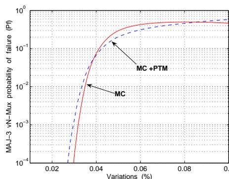
**Figure 3.** MAJ-3 vN-Mux Probability of Failure calculated using MC and hybrid MC-PTM simulations
