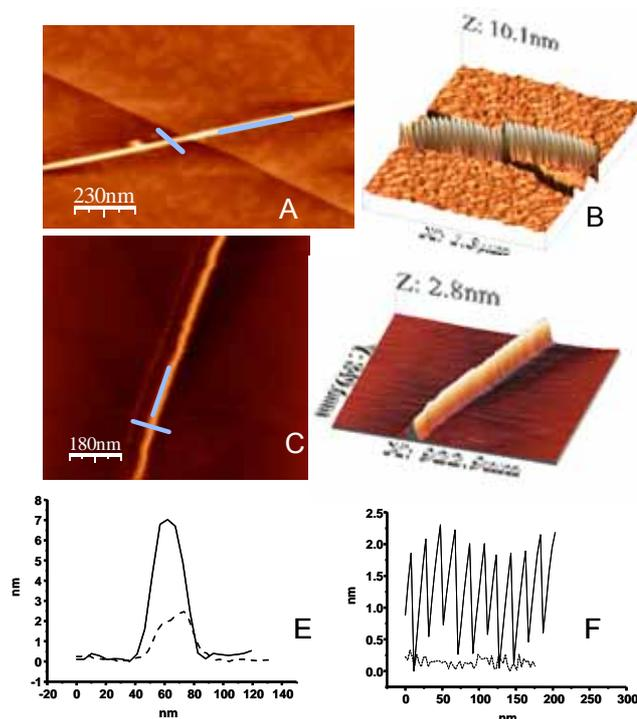
**Figure 2.** AFM characterization of the height and roughness of control MWCNT (panels C, D, and dashed line in panels E and F) and hydrogenase-coated MWCNT (panels A, B and solid line in panels E and F) deposited on highly oriented pyrolytic graphite.
