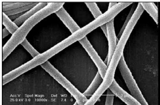
Fig.1. SEM micrograph of 10wt% of PANi (20 Kv)
