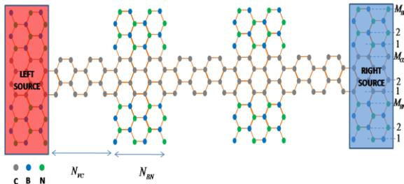
Fig 1: Studied structure with BN flakes attached to a graphene ribbon in the channel. We define  $n_{BN}$  as the number of BN/G/BN sections in the active region.
