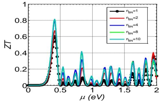
Fig 2: Figure of merit  $ZT$  as a function of chemical potential for different values of  $n_{BN}$ . The structure parameters are  $M_{CC}=5$ ,  $M_{BN}=9$ ,  $N_{VC}=N_{BN}=8$ . Simulation was performed at  $T=300$  K.
