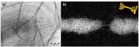
Figure 1. a) TEM and b) HAADF-STEM images of Au NWs. Single-atom thick chain formed during wire fragmentation under E-beam irradiation.
