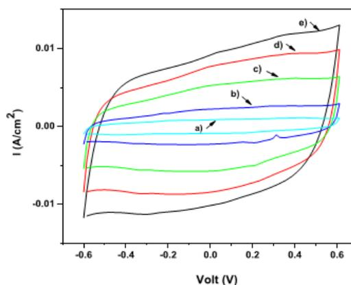
Cyclic voltammogram of PEDOT-MnO<sub>2</sub> composite in acetonitrile containing 1M LiClO<sub>4</sub> electrolyte at a scan rate (a) 2mV/s, (b) 5mV/s, (c) 10 mV/s (d) 15 mV/s and (e) 20 mV/s in a potential range between 0.6 and -0.6 V.
