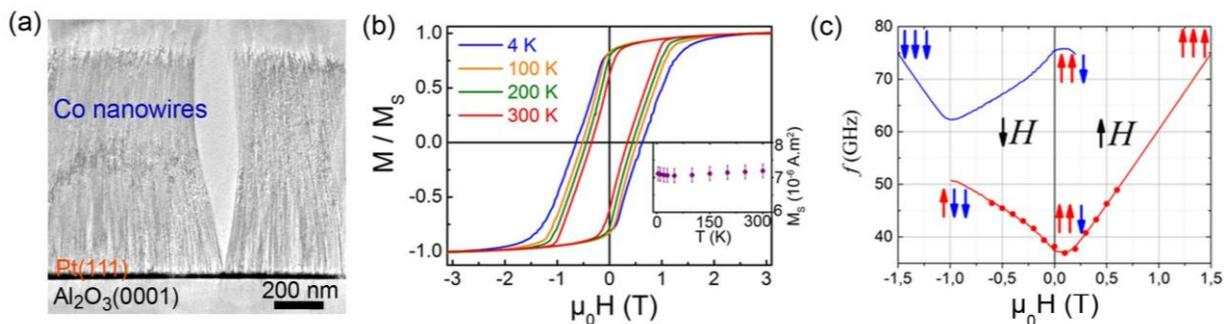
(a) TEM micrograph of a Co NW array grown on Pt(111)/Al<sub>2</sub>O<sub>3</sub>(0001). (b) Magnetic hysteresis loops measured for a magnetic field applied along the NW, *i.e.* the easy axis of magnetization. (c) FMR resonance frequencies as a function of the applied DC magnetic field (dots: measurements, lines: model).
