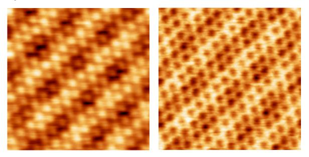
**Fig 1.**  $6x6nm^2$  simultaneously recorded atomic resolution NC-AFM images on Graphene/Pt(111); a) Topography image at a set point  $\Delta f = -72Hz$ . A hexagonal lattice with only one maximum per unit cell is observed; b) Simultaneously recorded image at a lower (in absolute value) set point  $\Delta f = -62Hz$  where a honeycomb pattern is detected. Both images were taken using the retrace technique with the WSxM software (8). Oscillation amplitude: 20nm, bias voltage: 0V.
