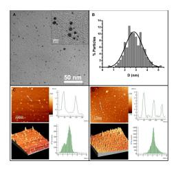
Characterization of VIP-gold nanoparticles. (A) TEM image of AuNPs, scale bar; 50 nm. The inset shows a higher magnification image, scale bar; 5 nm. (B) Statistical analysis of colloid diameter, as evaluated from TEM image. (C) TM-AFM image of tiopronin AuNPs and (D) TM-AFM image of VIP AuNPs.
